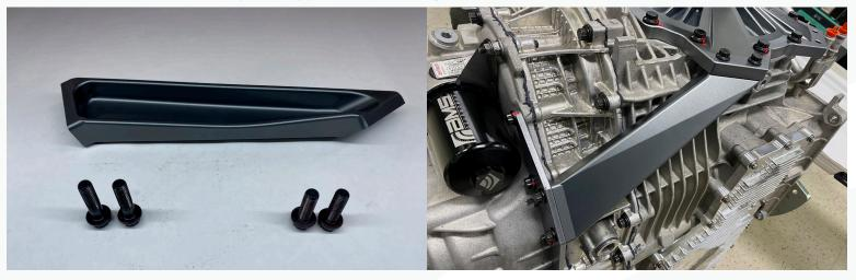
16. Locate the smallest support arm and 2 - m8 x 30mm and 1 – m10 x 70mm long bolt. The m10 bolt will need to be placed in the arm before installing the arm for the bolt to fit. Then slide the arm on the trans case and attach to the brace with the m8 bolts. **Torque the m8 bolts to 24 ft-lbs.**
