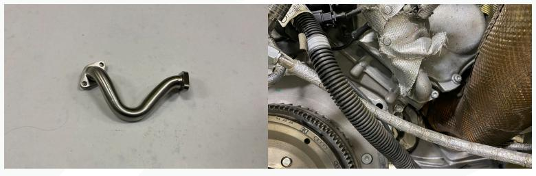
19. Unbutton the heat shield on the passenger side air valve to gain access to the fasteners. Remove the cast section of the tube and reinstall the provided relocation tube reusing the gaskets and hardware.
