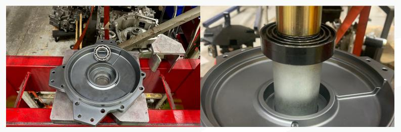
7. Once the bearing is fully seated, install the snap ring.
