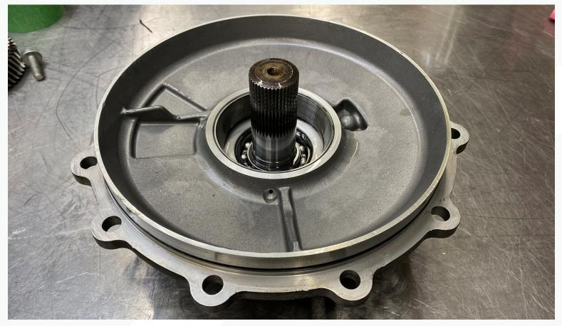
2. If you are upgrading the half shafts you do not need to remove the OEM half shafts to remove the race. If you choose to you can remove the snap ring shown in the 1st picture and press the shaft out.
