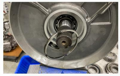
5. Locate the bearing, snap ring, and two seals provided and place them with the bearing race and spacer.
