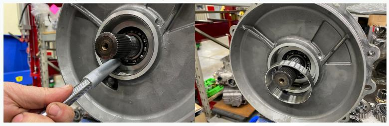
4. Remove the spacer and set it and bearing race aside for a later step.
