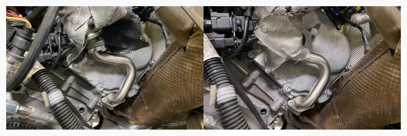
20. Reinstall the air valve pipe to the engine and resecure the heat shield.
