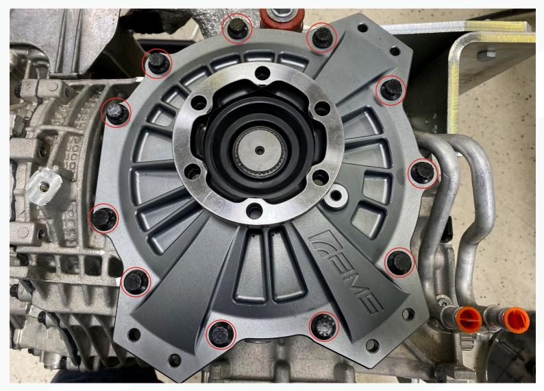
14. Locate the mid plate support bracket and 4 m8 x 30 ARP bolts. Install the bolts onto the rear cover by removing the existing hardware and replacing with the new ARP hardware. **Torque the M8 hardware to 24 ft-lbs**
