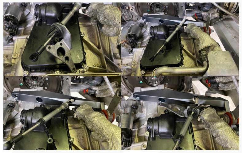
22. Reinstall the transmission. The torque specification for the hardware that mounts to the transmission to the engine is: M12:  $30NM + 45^{\circ}$ , M10:  $15NM + 45^{\circ}$
