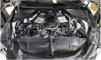
2. Loosen the two hose clamps (arrows), then remove the four intercooler bolts (circled). Two of the bolts are below the engine harness. See photo below.
