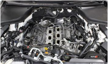
NOTE: If you have not already, clean up any debris in or around the valley of the engine. Any contaminants in the fuel system can lead to injector failure. Also, it is a good idea to use paper towels to plug the intake ports to keep debris from falling in while the manifold is off.
