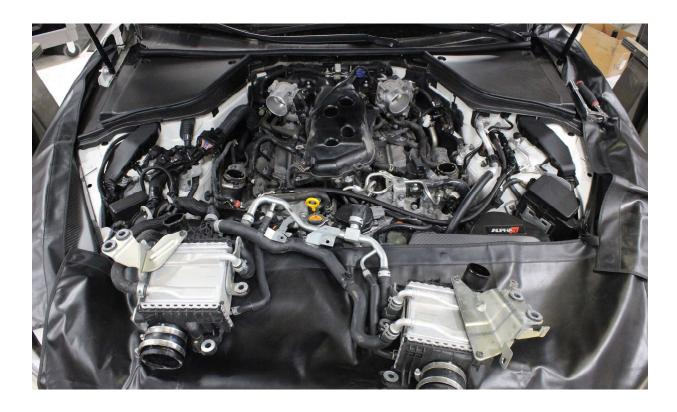
10.If you have hose pinchers, use them in this step to have minimal coolant loss and avoid having to re-bleed the cooling system. Pinch off both throttle body hoses and slide the outer most hose clamp back and remove outside hose as shown below.
