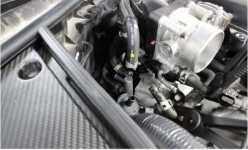
13. Using a long flat blade screwdriver, release the clip and pull the hose off the bracket.
