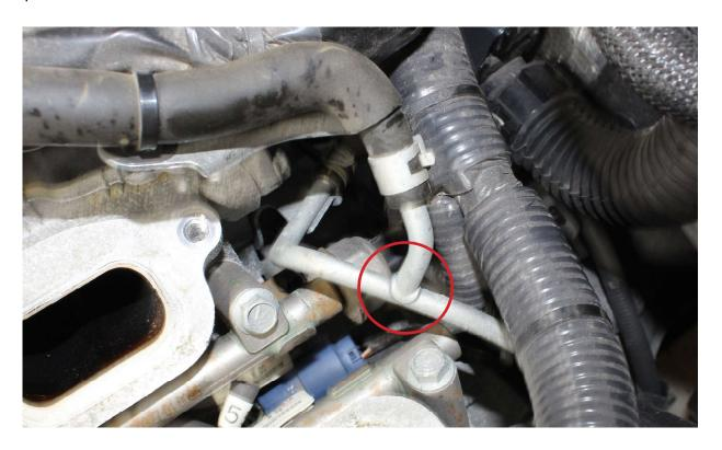
20. Due to the design of the fuel rails, the passenger rail needs to be remove first. Remove the two nuts and two bolts holding the passenger side fuel rail to the cylinder head. Work the rail free and remove it as shown below.
