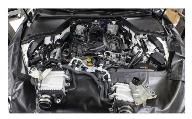
10.If you have hose pinchers, use them in this step to have minimal coolant loss and avoid having to re-bleed the cooling system. Pinch off both throttle body hoses and slide the outer most hose clamp back and remove outside hose as shown below.
