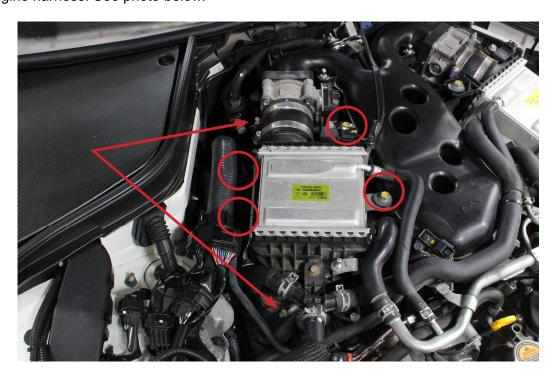
3. Disconnect the map sensor mounted on the intercooler.
