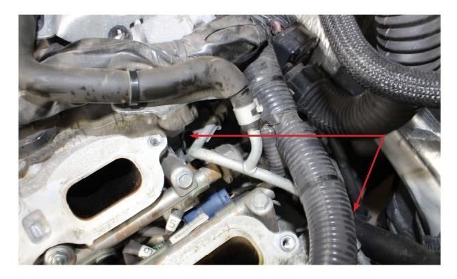
19. Disconnect the fuel pressure sensor connector and the black fuel injector harness connector just below the fuel pressure sensor.
