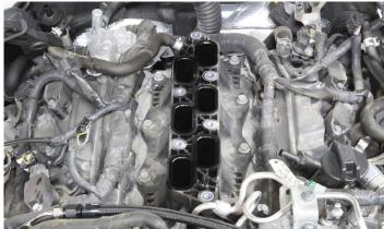
16. Remove eight lower intake bolts to remove the lower intake.
