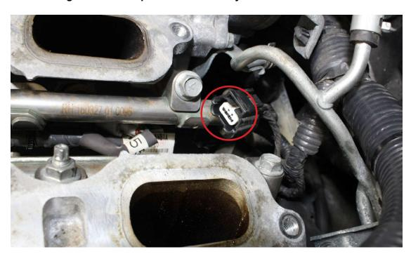
25. Apply a small amount of engine oil to the fuel rail inlet threads and reinstall the high pressure fuel line removed in step 17 by starting the nuts by hand on the rail and then the fuel pump. Install the bracket bolt before tightening the lines.
