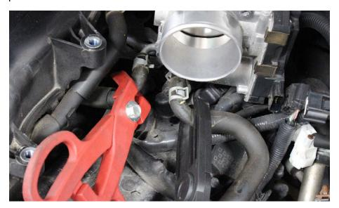
12. Remove the hose behind the intake manifold on the passenger side.
