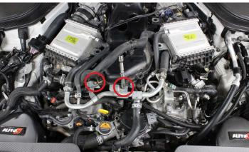
8. Lift at the front of one of the intercoolers to pull the intercooler out of the coupler, then pull it off the throttle body. Repeat on opposite side.
