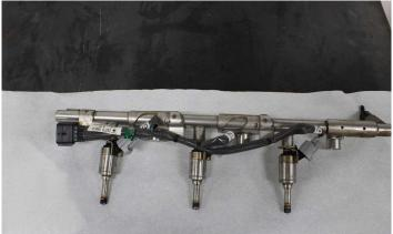
23. Replace each injector by disconnecting the connector and removing from the rail. Apply a small amount of O-ring safe grease to the new o-rings. Ensure that none of the grease ends up in the inlet of the injectors.
