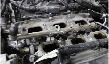
21. Disconnect the driver side fuel rail connector and remove the bolts holding the fuel rail. Remove the fuel rail.
