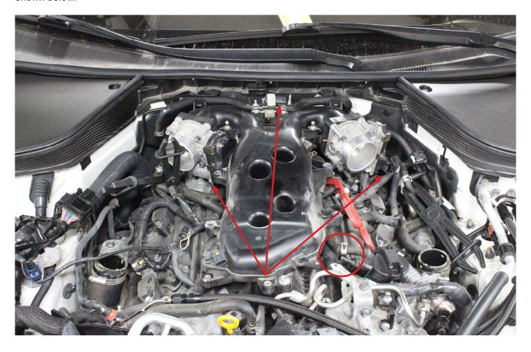
15. Remove the six upper intake manifold bolts. Then remove the intake manifold.
