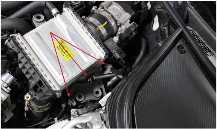
7. Disconnect the connector and release the clip to lift up the hose. Remove the two bolts underneath.
