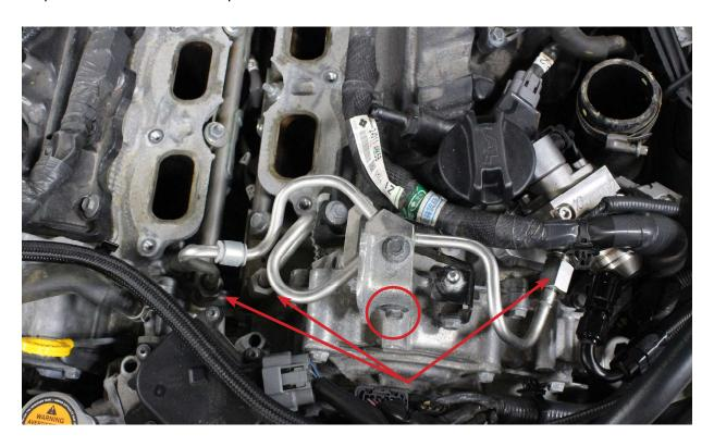
18. Remove the two bracket bolts holding the hard pipe on the back of the head to create more room to slide the fuel rails out.
