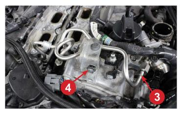
26. Reinstall all parts in reverse order. If you pinched off the coolant hoses to the throttle body, it is not necessary to bleed the cooling system.
