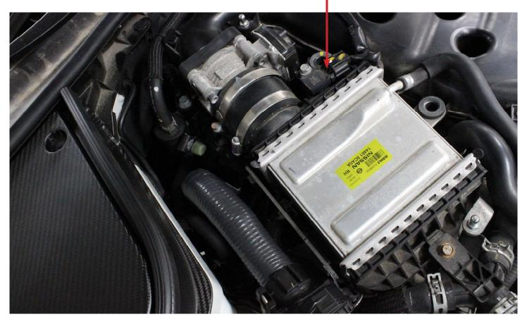
4. Disconnect the hose and remove the bolt holding the bracket.
