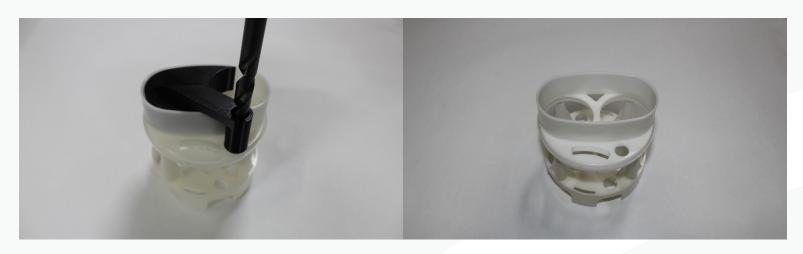
25. Gather the following parts – fuel pumps, filter pickups, O-rings and top & bottom caps. Starting with the top & bottom caps, notice two have a section machined out to create a light cinch feature (top cap) while two do not (bottom cap). Grab one of each and place an O-ring inside the groove as shown. This will be for the first pump.
