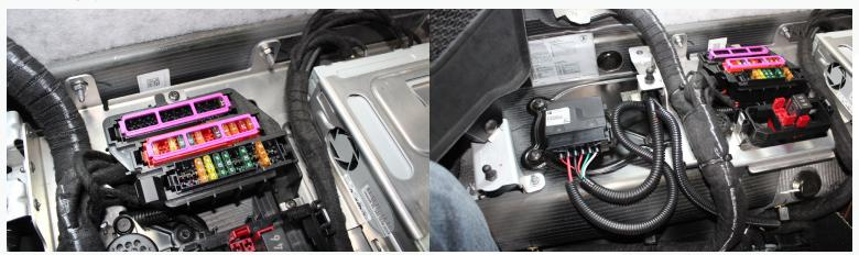
76. Locate the provided 30A fuse. Install it into the location where the wire was added. Reinstall the purple fuse cover.
