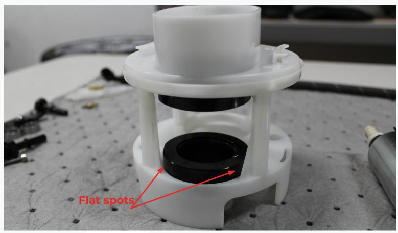
27. Lubricate the O-rings with a silicone spray or similar. Place the pumps into the basket until they sit all the way down while keeping the upper cap in position. Check that the machined flats are also in correct position. See photos for correct clocking of the pump outlet barb.
