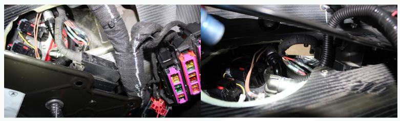
67. Reinstall both rear access panels, then reinstall the rear panel frame and components. If you opted to remove the fuse panel you can leave that out for now. Otherwise, if you did not, you will need to remove it for the next steps.
