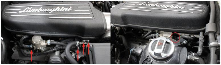
2. Disconnect the 2 connectors on the backside of the manifold near the firewall and the two throttle body connectors. We have shown a manifold off the car to help locate exactly where they are.
