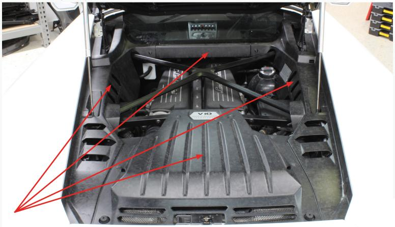
2. Route the hose installed in step 53 of the Alpha Dual Brushless in-tank instructions up behind the fuel tank heat shield past the coolant reservoir and to the driver's side engine bay area as show below.
