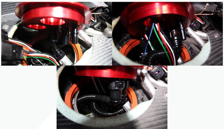
49. Pass the fuel pump harnesses through the opening before placing the top hat in place. Once the top hat is in place, it is a good opportunity to verify all internal lines and wires are not kinked or obstructing level sensor operation. Once verified, reinstall the top hat nut.
