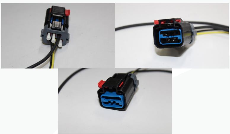
62. With the loomed harness through the grommet, insert the terminals in the orientation shown below. Then reset the secondary pin lock.
