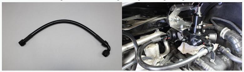
16. Locate the three fuel lines. The longest one goes from the further most #6 port to the passenger fuel rail. The next line (middle) is the next fitting on the regulator and connects to the driver's side rail. The last line (heat wrapped) connects to the last port and the fitting on the intake manifold.
