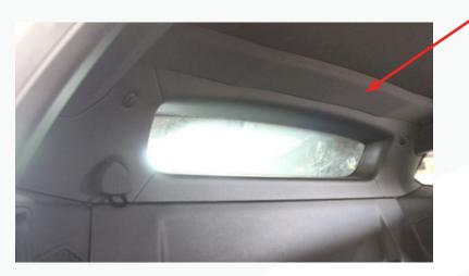
9. Remove the plastic cover to reveal the bolt holding the child seat hook. Then remove the window trim plastic.
