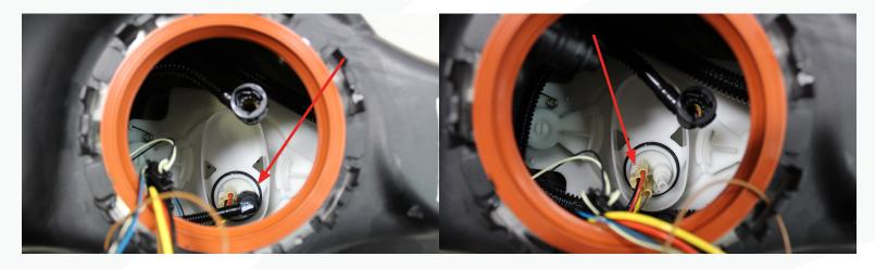
20. Flip the two levers shown remove the fuel sending unit and place it on your workbench.
