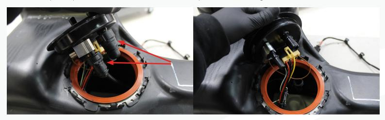
19. In the tank, disconnect the fuel line off the pump and the electrical connector.
