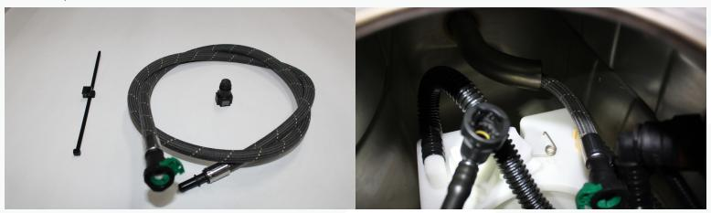
37. On the driver side tank, route the line away from the level sensor by leaving a little slack in the line and wrapping around the backside of the sensor with the zip tie mount. Then make the connection as shown in the last photo below.
