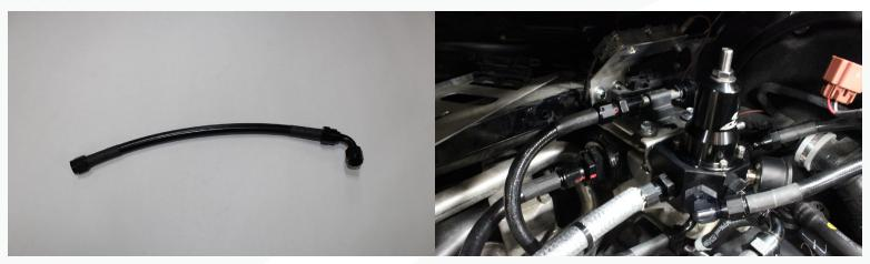
22. Install the longer of the two lines from the flex fuel connection over to the quick connect fitting installed in step
