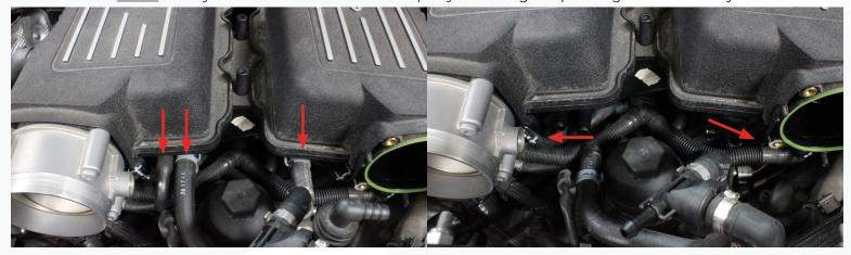
4. Disconnect the 90° vacuum connection below the passenger side fuse box. Then remove the 5 bolts holding on the center intake cover and remove the twelve T30 intake manifold mounting bolts. Remove the manifold.
