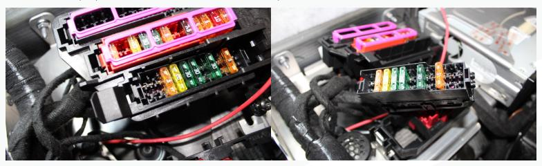
73. Flip the fuse rail over and remove the cover. Notice the purple terminal lock, this needs to be removed in order to insert the new pin. Using a small flat blade screw driver, you can push it out from the backside.
