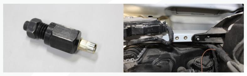
7. Using the two m6 bolts and washers, install the bracket on frame. If the vehicle had the antenna mounted there, mount both brackets on the frame sandwiching the new bracket as shown below.
