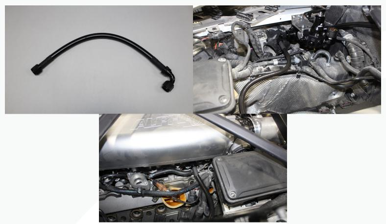
17. Locate the (3) fuel lines. The longest one goes from the further most #6 port to the passenger fuel rail. Connect the middle line from the angled port on the regulator to the driver's side rail. The last line (heat wrapped) connects to the last port and the fitting on the intake manifold.
