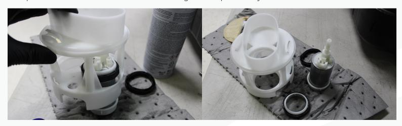
24. Using the empty basket, locate the 3D printed drill jig and set it in the top of the basket in such a way it covers the open hole. This will locate the holes to be drilled. Using a 2" hole saw and a 14mm (or similar) drill bit, drill the two holes as shown below. Remove any burrs or debris.
