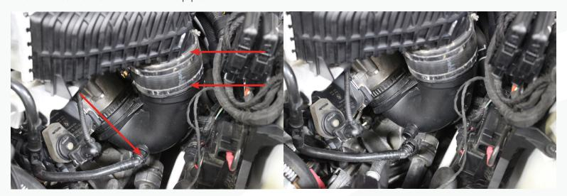
4d. To remove the pipe from the throttle body, you will need to remove the white retaining clip. The following pictures show the clip and its location.
