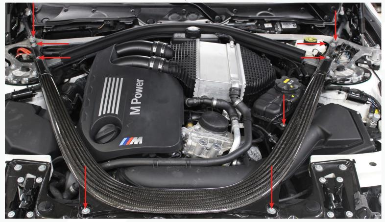
3. Begin with the right airbox (passenger side), disconnect the MAF sensor from the airbox and loosen the worm clamp using a 6mm socket. Remove the coupler attached to the airbox and push out of the way. Remove airbox by pulling up on the box to release to from the three mounting grommets. Set airbox aside.
