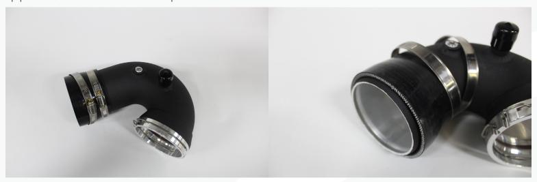
6c. Remove both O-rings from the stock right (passenger side) charge pipes, and transfer to the AMS pipes. Now install the silicone couplers onto both pipes also slide on two worm clamps onto each pipe as shown below.
