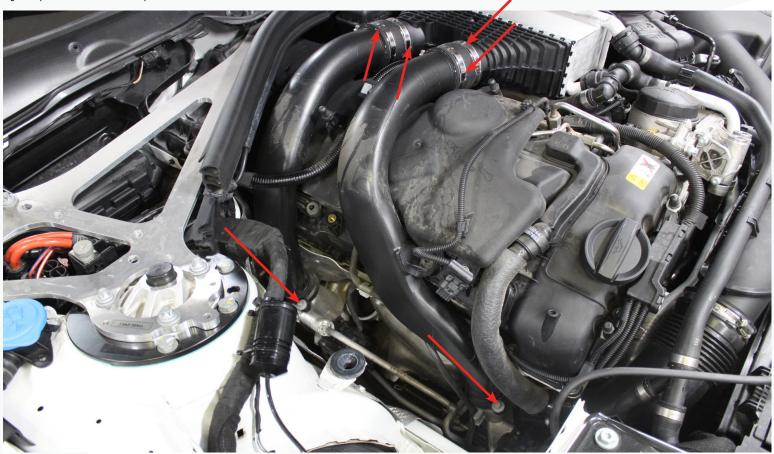
4a. To remove the plastic turbo inlet tube, remove 10mm bolt and pull out the tube. There is a rubber O-ring on the inlet. Make sure this remains in place, as it will be reused.
