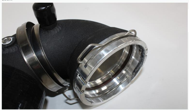
6a. Slide the pipe onto the throttle body and attach the retaining clip as shown.
