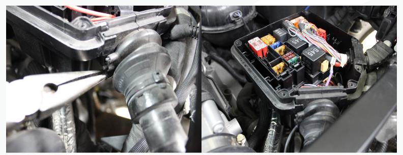
14. Next, grab the single black wire from the water pump wire harness kit. Feed the non-insulated end into the fuse box next to the purple wire. Route the other insulated end down to the pressure switch just below the boost controller. Secure to the engine harness with zipties.
