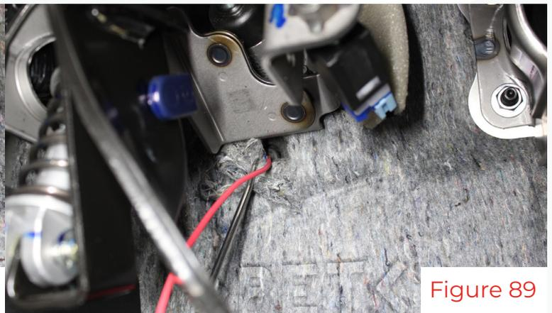
39. Pull the red wire through to the cowl compartment(fig 90) and begin running the wire under the cowl cover and over to the Zeitronix module(fig 91 & 92).
