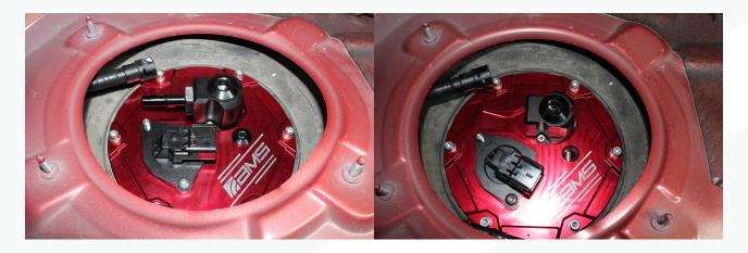
a. Install the provided 8AN to 6AN outlet fitting into the outlet block and the swivel quick connect fitting into the top hat.
