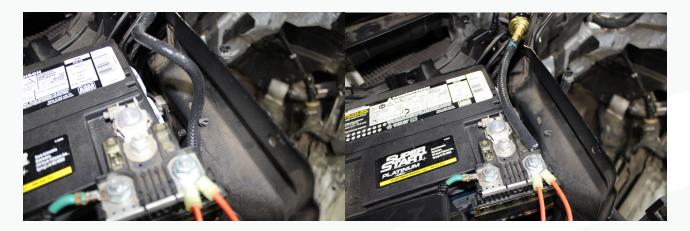
119. Install the straight barb fitting with a clamp and point the other end through the hole. Connect the remaining hose to the barb on the opposite side of the firewall and clamp it.
