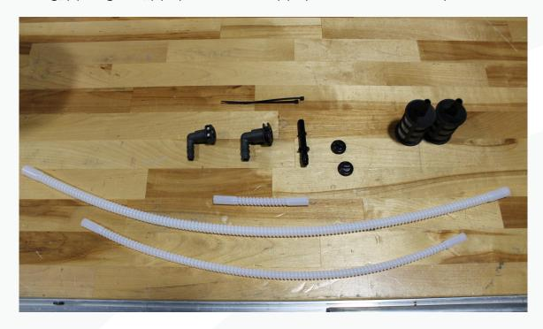
50. Assemble the small siphon adapter hose using the 5/16 90 degree quick connect fitting, siphon hose and adapter fitting. Carefully apply a little heat to the end of the hose using a heat gun to fully seat the siphon hose. **Caution:** Too much heat may permanently damage the hose. Install the <u>green quick connect</u> clip on the siphon adapter.
