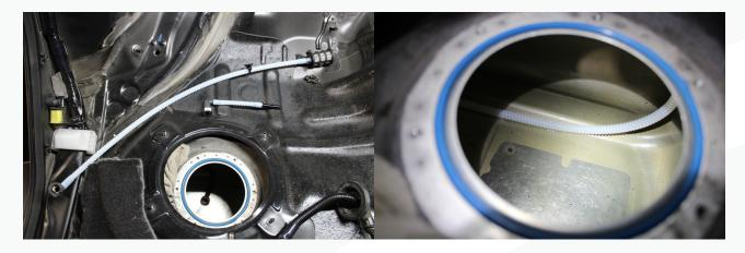
59. Place the new bottom basket into the tank followed by the upper basket. Match up the alignment tubes on the inside of the basket, they only match up one way.
