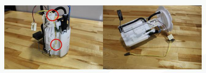
14. Push the level sensor retaining lock over and slide the sensor up and out. Set it aside for later.
