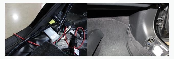
99. Starting at the b pillar, slide the split loom over the red and black wires towards the relay.
