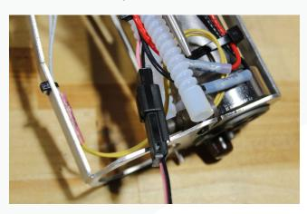
43. Cut off the OEM level sensor connector about an inch away from the connector.
