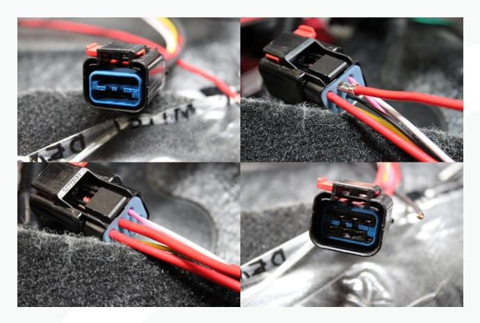
89. Put a 180-degree bend in the green and brown wires and then bundle the group of wires together. Starting from the OEM loom, wrap the wiring with electrical tape up to the T. Then place a section of electrical tape near the 180-degree bend to hold the other bundle in place.
