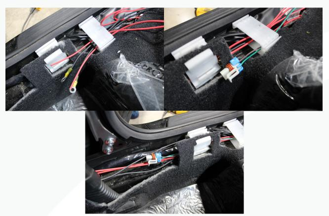
96. Locate the chassis ground on the b pillar above the seat belt retractor and install the ring terminals.
