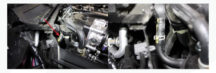
122. Place one more clamp on the small section of hose, then push the open barb onto the hose that was just removed and clamp it. Then install the new hose on the intake manifold barb and tighten the clamp.
