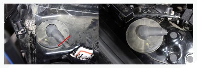
104. Feed the wires up through the hole into the battery compartment. Then while holding the grommet, feed the wires and loom through the grommet at click the grommet back in place.
