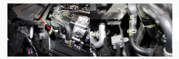
111. Place one more clamp on the small section of hose, then push the open barb onto the hose that was just removed and clamp it. Then install the new hose on the intake manifold barb and tighten the clamp.
