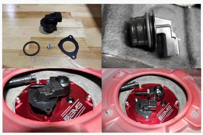
72. <u>Option 1 Dead Head/Returnless</u> - Install the white quick connect removed earlier onto the top hat fitting. Hook the factory line to the top hat.
