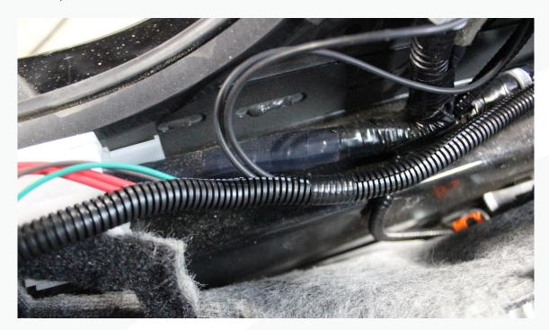
101. Continue feeding the harness in the loom. Once the whole harness has been loomed, feed it through the rest of the harness retainers along the sill.
