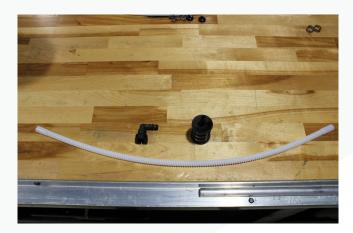
52. Assemble the hose as shown below, using the cinch clamp on the siphon strainer. Again, using a small amount of heat without damaging the hose, affix the 3/8 quick connect fitting to the other end of the siphon hose. Measure 6" from the strainer, fix the magnet to the hose with 1 zip tie.
