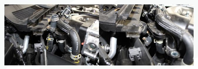
112. Locate the round sticker covering the hole near the battery. This hole will be large enough to pass our vacuum hose through. Remove the sticker.
