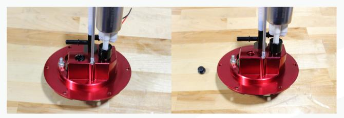
20. Grab the fuel pump, fuel pump grommet, and fuel pump fitting. Lubricate the grommet inside and out, then install it into the fitting. Then lubricate the O-ring and install the fitting in the open port.
