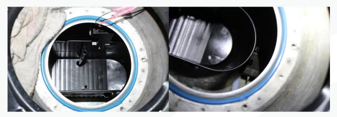
65. Set the basket near the opening in the fuel tank and connect the level sensor.
