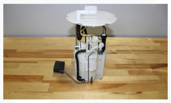
12. Disconnect the two electrical connectors.
