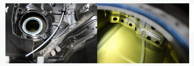
56. Instll a 11.3 Oetiker clamp onto the end of the hose and push the open end of the hose onto the metal tube at the front of the tank. Cinch the lamp with Oetiker pliers to secure the line to the tube.
