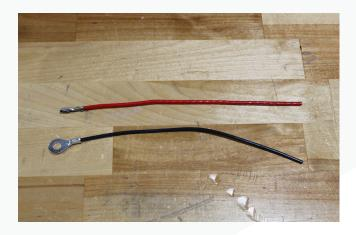
36. Install the pinned red wire into the open cavity next to the other red wire on the connector.
