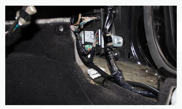
106. Locate the (2) orange fuse holders, (2) ring terminals, (2) butt connectors and (2) large heat shrinks. Strip the ends of the fuse holder and install a ring terminal at one end and butt connector at the other. Slide the heat shrink onto the butt connectors.
