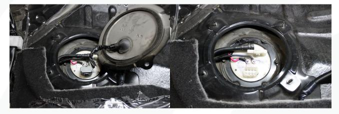
**Note:** This vehicle has another aftermarket system installed which you can see by the two extra eyelet connections on the top hat. This system will be removed during installation of the AMS Race X LSFP.
