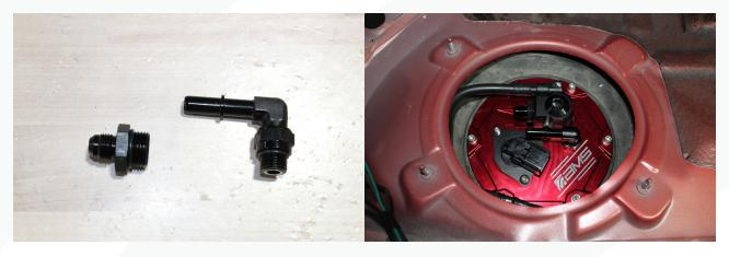
b. Install the white quick connect clip removed earlier onto the top hat fitting.
