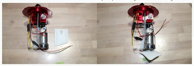
33. Using one zip tie, attach the section of wire to the side of the hanger. Put retainer side of the zip tie on the inside as shown below.
