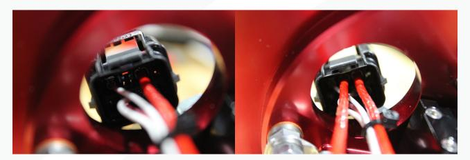
37. Remove the ground nut from the top hat and install the second ground wire. Position the two eyelets back-to-back and tighten the nut. Be sure to clock them down so they are almost touching the top hat but out of the way of the connector hole in the top hat.
