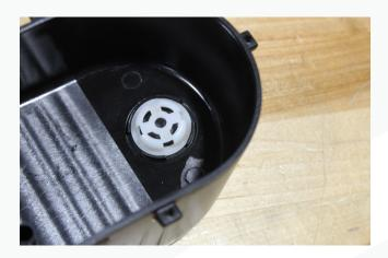
48. On the side of the basket there will be two dimple features. The Q50/60 you will need to drill the top hole with a 13/64 drill bit. On the Z the basket has three tiers, so you will need to drill both the holes on **only** the top tier.
