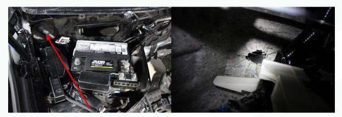
103. Trim the grommet indicated by the red line below just before it enlarges. This spot will fit tight on the loom to help prevent leaks.
