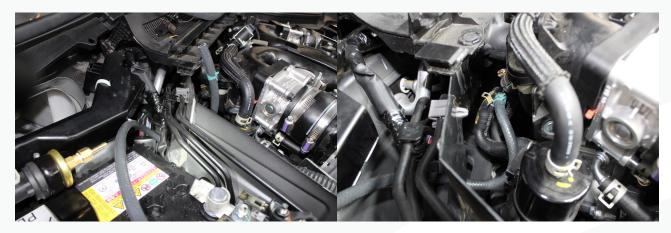
114. Route the hose with enough slack for engine movement back to the hobbs switch on the battery. Trim the hose and secure it with a clamp. **Then skip to step 124.**
