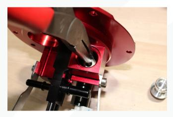
3. Locate the provided dummy plug. Place a little lube on the o ring and install it in place of the regualtor.
