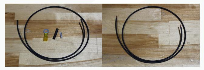
94. Crimp the (2) black ground wires made in the previous step to the unterminated black wires coming from the 2 pin connectors.
