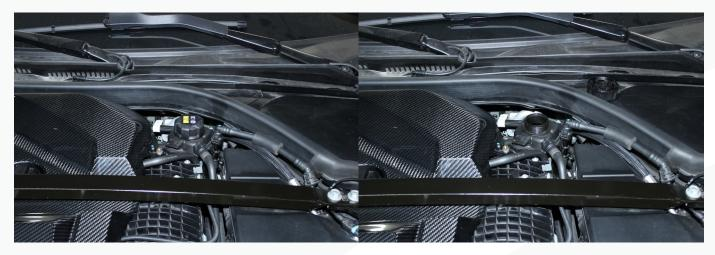
6. Remove the (6) clips from the top bumper garnish and set the garnish aside.
