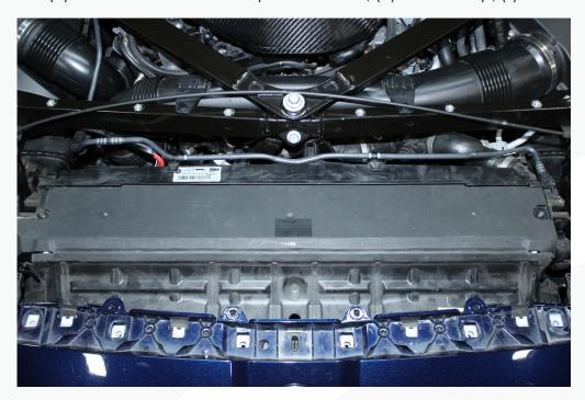
12. Release the tab on the side of the fan assembly and lift it up about a half an inch. Then release the clip on the plastic cover and remove the cover.
