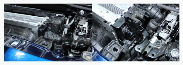
14. There is a small retaining tab on the driver's side of the HX that you can see through the front grill. With a small screwdriver, push that tab in and lift up on the HX. Once the tab is passed the hole you can lift the HX up and out.
