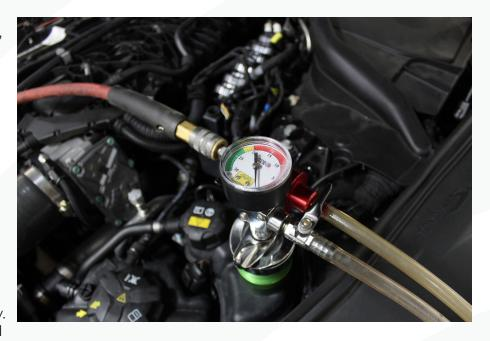
filling procedures will not work for this application. The method we prefer uses a widely available system called an Air Lift or Vacuum Venturi System. These systems use compressed air to draw the cooling system under a vacuum and remove all the air from the system. The vacuum then draws in coolant into the entire system. Almost no bleeding is required after.
