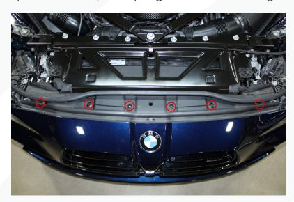
7. Remove the bolts securing the front bumper and the (3) bracket bolts.
