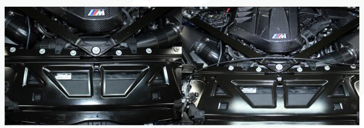
10. Remove (6) hex, (4) T40, and (2) T30 bolts. Remove the radiator support cover and set it aside.
