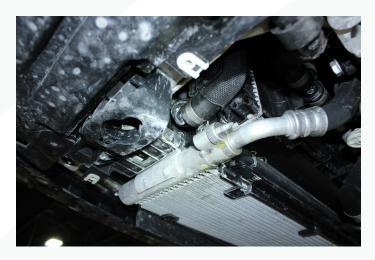
4. With the engine cool, carefully disconnect the lower heat exchanger hose by releasing the metal clip and pulling down. Use some silicone spray or penetrating lubricant and aim into the top of the plastic fitting to assist with stubborn ones. Let it drain while you work on the top side.
