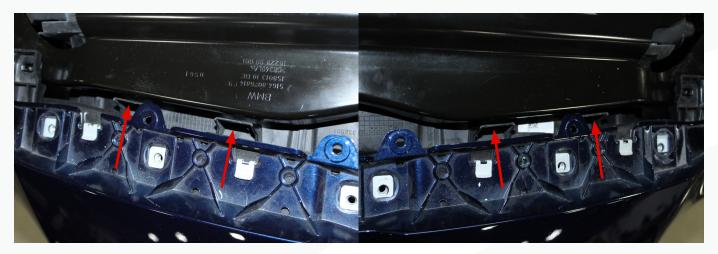
9. Remove the cable from the (3) metal clips and position the cable out of the way or remove the cable from the passenger side latch.
