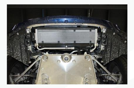
3. Locate the lower heat exchanger fitting and place a coolant catch can underneath.
