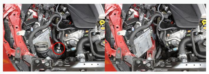
9. For the right side only (Passenger Side), remove the OEM air box support bracket.
