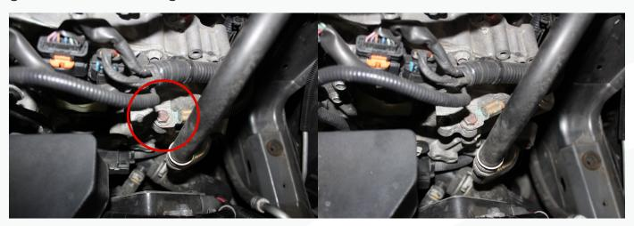
17. It's easiest to test fit the intakes without the filter and mark the position of the MAF on the bracket to then assemble the intake assembly out of the car. Having the MAF in the correct position is very important to the performance of the intake.
