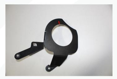
**21.** Position the brackets on the bench like they would be installed on the car. Install the filters through the top of the bracket with the logo on the filter facing forward.
