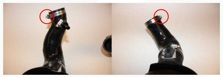
**24.** On the passenger side, plug in the MAF sensor and install the vacuum hose to the barb fitting. Then install the intake onto the turbo.
