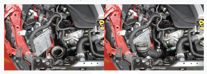
**8.** Disconnect the PCV hose from the OEM coupler. Only disconnect the small clamp at this time. Completely remove the OEM coupler.
