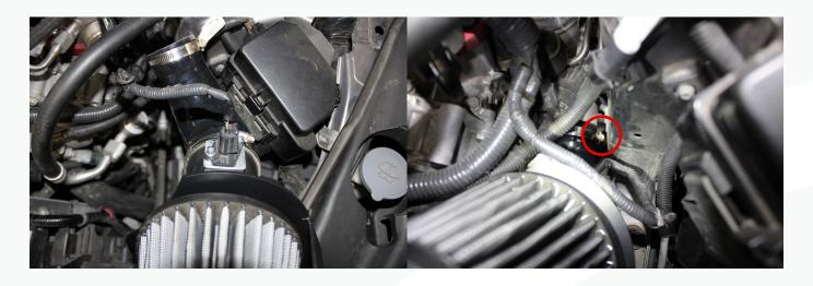
**26.** Once the clamps are tight, install the (4) M6 intake mounting bolts.
