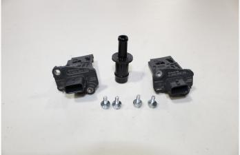
**11.** Locate the new MAF housings and install the MAF sensors into the housing. Be sure the arrow on the MAF flange matches the arrow on the sensor.
