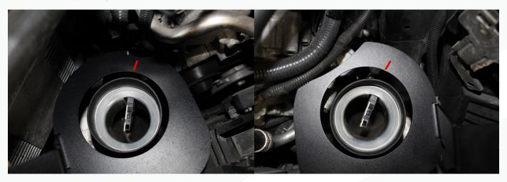
**20.** Place the brackets on the bench, transfer the mark you made onto the underside of the bracket.
