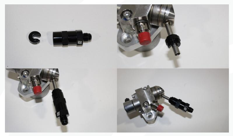
4) Reconnect the removed fuel line and check for leaks by cycling the key a few times before starting.
