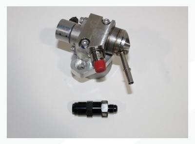
3) Remove the locking collar from the quick connect fitting and install it onto the collar on the pump inlet. Slide the fitting onto the pump and screw on quick connect collar and tighten with two wrenches.
