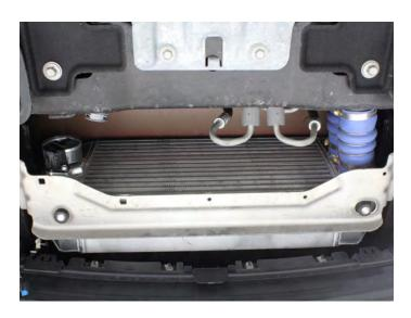
15. Install the new intercooler outlet coupler using the provided hose clamps. The outlet coupler will only install in one direction. The outlet on the intercooler and the OEM charge pipe are different sizes.
