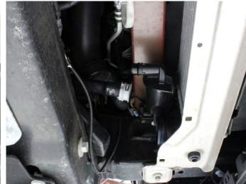
**06.** Unbolt the lower intercooler mount from both sides of the frame. Carefully lower the intercooler down to gain access to the bypass valve wiring harness. This harness may be a little tricky to remove. The harness is held in place by two fir tree style clips into the top of the intercooler. Release these clips and remove the intercooler. Below is a picture of the harness and intercooler removed from the truck to give you an idea of what is going on.
