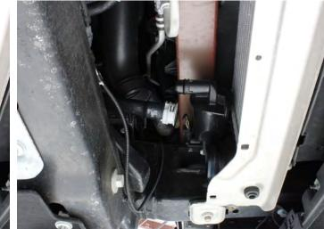
**04.** On the passenger side, remove both OEM blue intercooler inlet couplers. Save these couplers as they will get reused during the AMS Intercooler install.
