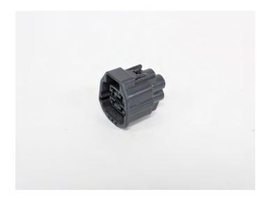
**21.** Insert the four terminal plugs into the rear of the connector.
