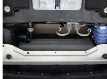
**02.** On the driver's side, disconnect the bypass valve hose connection from the intercooler. Turn the grey connector counter clockwise to release the connection. Next, remove the OEM rubber coupler from the intercooler outlet. The OEM coupler will not get reused.
