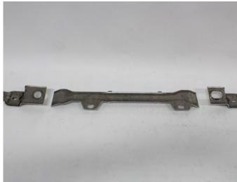
**10.** Discard the center part of the upper intercooler support. Reinstall the two ends using the supplied longer bolts and spacers.
