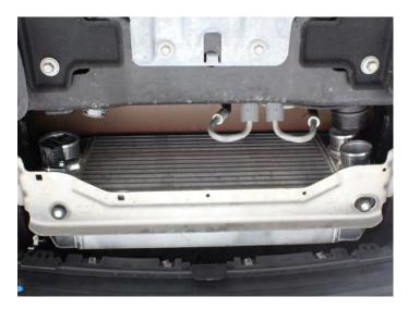
**14.** Reinstall the OEM blue intercooler inlet couplers.
