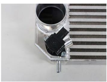
12. Remove the four rubber intercooler mounts from the OEM intercooler and transfer them to the AMS Intercooler.
