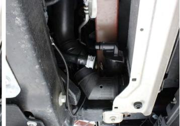
**03.** Remove the plastic elbow from the intercooler. Do so by releasing the metal retaining clip from the elbow.
