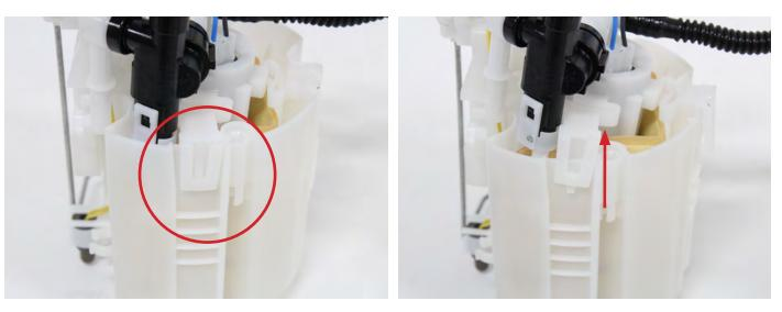
**16.** Remove the pump assembly from the sending unit basket.
