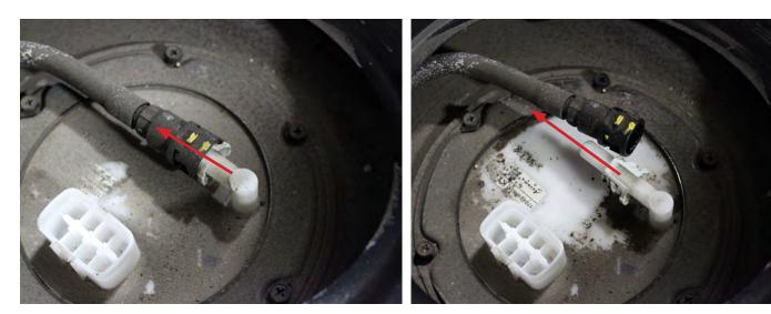
7. Clean the top of the fuel sending unit and fuel tank prior to proceeding. Cleanliness is important as to not introduce contaminants into the fuel cell.
