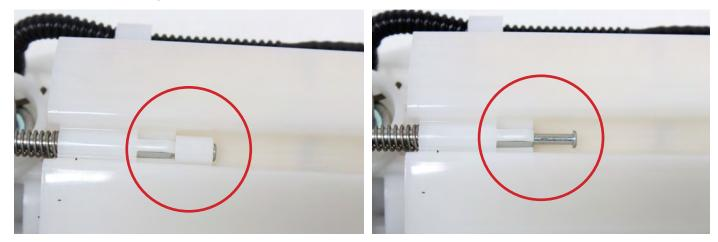
**12.** Release the tabs on both sides of the sending unit to release the spring loaded mounting rods.
