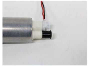
**23.** Place the O-ring from the factory pump onto the upgraded pump.
