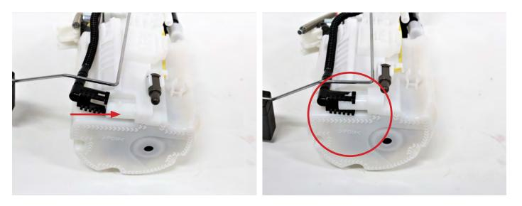
**34.** Cut the factory pump wiring about 2 inches from the white/clear pump connector. Strip the insulation from the ends of the blue and black wires on the harness remaining in the pump assembly by about 3/16".
