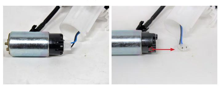
Check to see of the pump outlet O-ring removed with Remove the O-ring and set it to the side.
