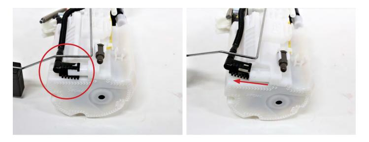
**15.** Release the 3 locking tabs securing the pump assembly to the sending unit.
