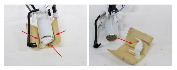
**18.** Remove the pump from the pump assembly.
