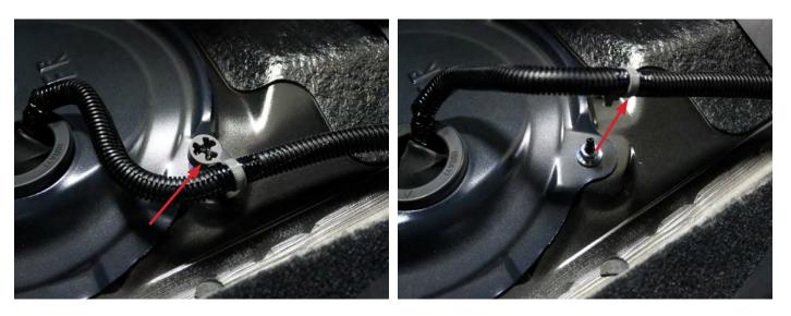
4. Remove the fuel pump sending unit cover by removing 3 - M6 nuts (10mm wrench).
