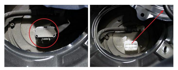
**6.** Make sure the fuel pressure has been relieved. Then disconnect the fuel hose connection on the top of the sending unit. Cover the connection with suitable rags to prevent fuel spray and to collect remaining fuel which may drain from hose.
