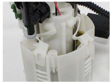
**31.** Reinstall the sending unit top hat. Reconnect electrical connections.
