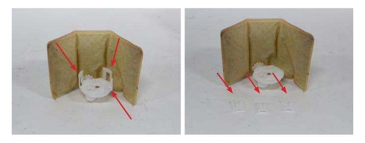
26. Locate the Alpha fuel pump bracket supplied in your kit. Note how the pump bracket fits onto the filter.
