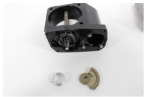
19. Install the smaller set screw into the location shown. This set screw is used to set fully closed position of the throttle plate.
