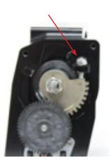
21. Now install the resting position set screw. This screw sets the resting throttle plate position. **Important: The final position of this screw must be set by your tuner.** To get a baseline, turn the screw in until it touches the stop cam or you feel the throttle plate just start to move from fully closed. Then Turn the screw 2 full revolutions clock-wise. Lock the screw down with the lock nut.
