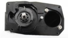
12. Check the rotational position of the throttle shaft. The "flat" of the shaft where the throttle plate secures to, must be facing outward. Outward can be determined by orienting the throttle body in a position that the "AL-PHA" engraving on the top of the throttle body can be read.
