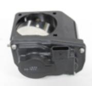
23. Install the Alpha endcap. Use green sleeve retaining compound on the mating edge of the endcap. Align and drive into place with a plastic or soft mallet.
