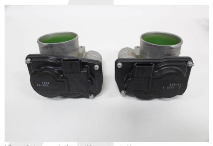
2. Remove the 4 screws per throttle body which secure the motor drive covers.
