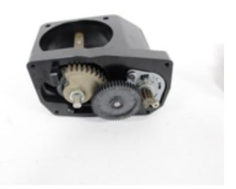
16. Insert the throttle plate into the throttle body housing. Make sure the throttle plate and housing are both facing a direction in which "ALPHA" can be read.
