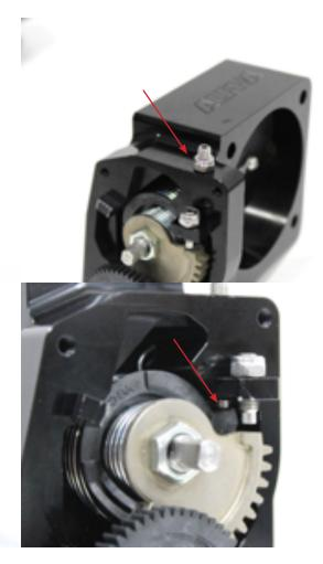
22. Reinstall the motor drive cover. Tighten the 4 screws securing the cover.
