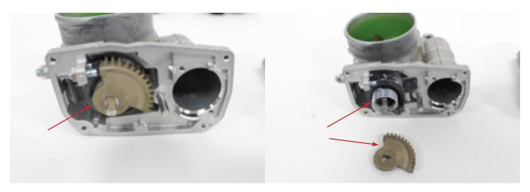
9. Remove the throttle stop cam. Pay close attention when removing. This stop cam is under spring tension. Note how the tension is applied. Remove the spring underneath and set both to the side.
