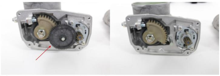
6. Remove the two screws securing the Drive motor. Remove the motor.
