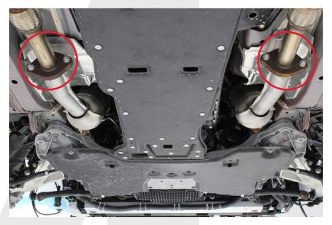
3. Loosen, but do not completely remove the lower downpipe mounting bolts. These will be completely removed when the downpipe is fully unbolted. Leaving the bolt in place will support the downpipe when it is fully unbolted.
