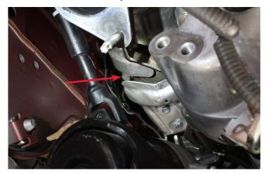
11. With a long extension and a swivel socket, completely remove the clamp bolt. Passenger side is similar.
