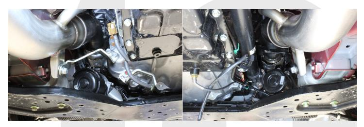
15. Connect the downpipes to the rest of the exhaust system with supplied hardware.
