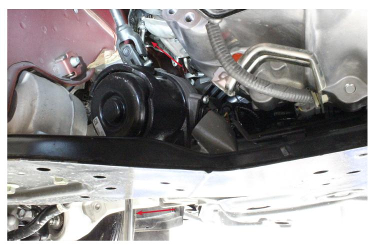
12. Completely remove the upper pipe support bracket. This will not be reinstalled. Passenger side is similar. There is also a slight difference between AWD and RWD vehicles on the passenger side.
