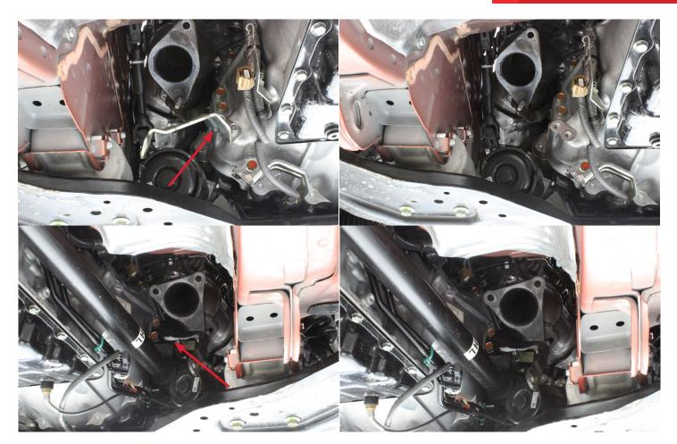
10) In order to get to the OEM band clamp, you need to loosen or possibly remove some of the heat shield bolts in order to move it out of the way. This is for gaining access to the V-band clamp. Repeat on opposite side.
