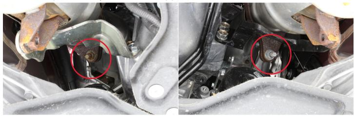
8. Transfer over the secondary O2 sensors to the new downpipes.
