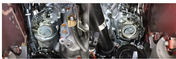
14. Install the new full downpipes using the same OEM clamp. It is recommended to use a little anti seize on the V-band bolt before reinstalling.
