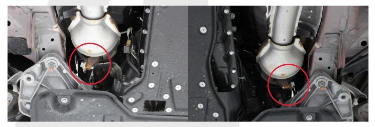
4. Disconnect the secondary O2 sensors. On the left side, the connector is located on the side of the transmission. On the right, it is located on the main engine harness just above the bell housing of the transmission. This connector is a little difficult to get to on AWD vehicles due to the forward shaft. You may need to completely unbolt the OEM downpipe first and move it to the side to gain access to the area. The picture below shows the connector on a RWD vehicle.
