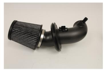
**10)** Now using the carbon air box, carefully slide the filter into the large hole of the air box and slide the isolator around the edge to create a seal as shown.
