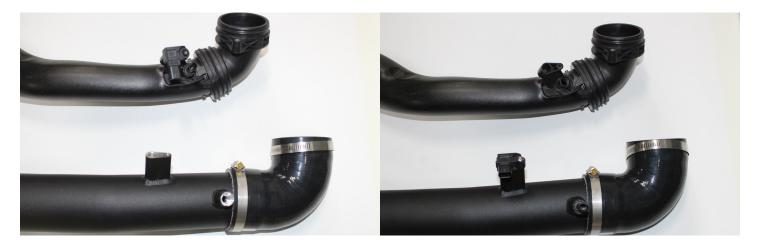
16. Slide the lower end of the charge pipe into the silicone coupler on the compressor side and push the upper silicone onto the throttle body. It will take some adjusting to get the pipe to sit correctly in the silicone couplers before you can tighten the hose clamps.
