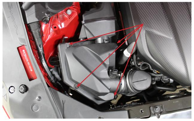
3. There are three grommets holding the air box in. One on the side and two underneath. Grab ahold of the lower airbox assembly and pull it straight up out of the grommets one at a time.
