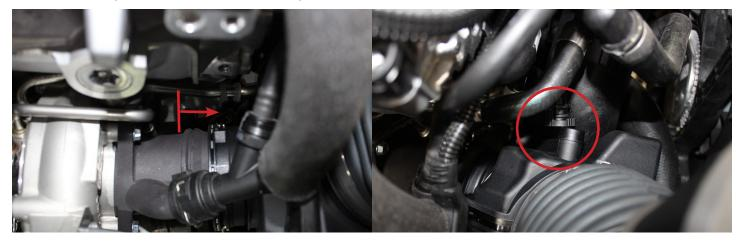
7. Unplug the two sensors on the charge pipe near the throttle body. Pull the white tabs out and press down while pulling on the connectors to remove them.
