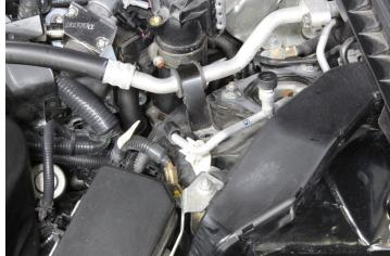
6) Use the supplied M6 x 22mm long button head bolt and install the flex fuel sensor and mount on top of the A/C bracket as shown.
