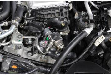
17) Locate the remaining 5/16" fuel line adapter fitting and install it on the HPFP. This fitting will work with the OEM HPFP and AMS HPFP. It does not get used on the AMS Big Bore HPFP.
