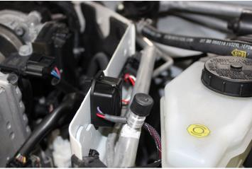
26) Remove the battery to gain access to the IPDM, if this has not already been done. Unclip the IPDM from its mounting bracket by releasing the two tabs at the top, then slide the IPDM upwards to remove from the bracket. To remove the cover, release the two tabs at the bottom of the IPDM cover, pull the bottom of the cover away from the IPDM slightly, then remove by lifting it upwards.
