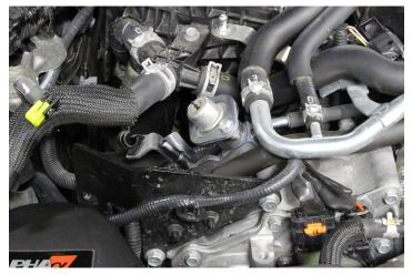
10) Unbolt the fuel line bracket from the engine. It is held in place by two M6 bolts located behind the black bracket shown.
