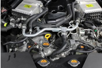
12) Locate the new low-pressure fuel line bracket. Swap the plastic fuel line clip from the OEM fuel line to the new bracket in the same orientation.
