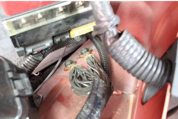
32) Now we will be adding a flex fuel input wire to the ECM. Ensure the battery is still disconnected. Locate and disconnect all three ECM connectors starting with the smallest connector and working your way towards the engine. They need to be disconnected in this order.
