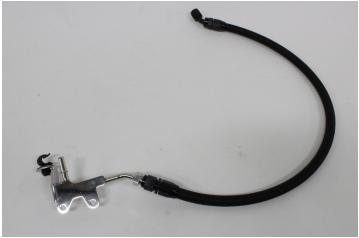
14) Install the new fuel line and bracket as shown under the intercooler water pipe. Once in place, reinstall the two M6 bolts holding water pipe to the intercooler.
