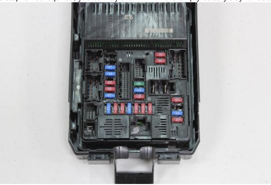
28) Locate the mini ATM fuse tap supplied in the kit and the supplied 10amp and 5 AMP mini fuses. Install the fuses as shown. It is important that the 10 AMP fuse is in the bottom and the 5 AMP be installed in the top. The bottom fuse location on the tap is for the fuse removed from the IPDM and protects the OEM circuit. The 5 AMP fuse specifically protects the circuit you are wiring, completely independent of the original fuse.
