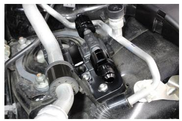
7) Remove the bracket in front of the HPFP. Unclip the harness and fuel line from the bracket. Unbolt the two 12mm bolts from the lower area of the bracket and remove. This bracket will not be reused.
