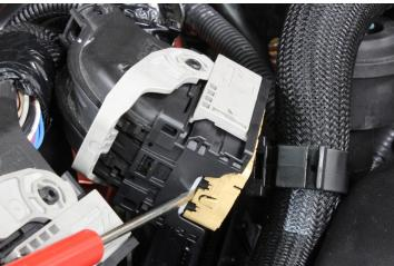
34) This step we will need to remove the cap and lever portion of the connector. Cut off the zip tie on the rear of the cover. Using a small flat blade screwdriver, remove cover and lever by releasing the retaining clip like shown the picture.
