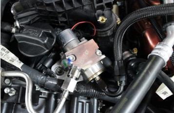
20) Double check all your connections. Reinstall the fuse removed during the first section of the instructions to relieve the fuel pressure. Key the car on a few times without starting it to prime the fuel system. Recheck all your connections for leaks.
