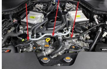
15) Reattach the fuel line to the new bracket as shown on the right side of the engine. Make sure the OEM fuel line is properly clipped into the plastic bracket.
