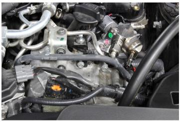
9) On the right side of the engine, disconnect the low-pressure fuel line from the bracket on the engine as shown.
