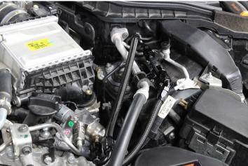
19) Alternately, if using the AMS Big Bore HPFP, the inlet fitting on the pump is a male -6AN. Attach the 180-degree fitting to the flex fuel sensor and the 150-degree fitting to the fuel pump.
