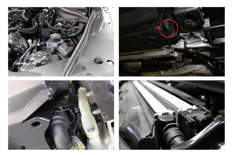
5. With both fittings removed, the factory heat exchanger can be lifted out.
