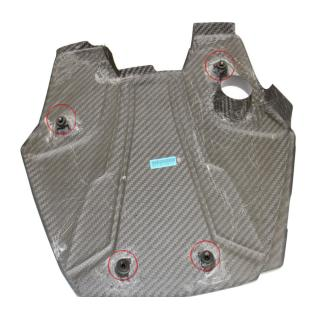
4. Remove the six 3-prong clips from the front and two 4-prong clips on the back corners of the cowl cover. Once removed, the lower half will need to be unscrewed and attached to the new carbon piece using the original screws.
