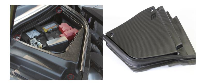
6. With the battery and brake covers removed, you can now remove the fender panels. These are held in place with five clips on either side and will require some prying to remove. Use a long panel clip tool and make sure you are prying around each clip. The clips will not be reused but the rubber seals will need to be transferred to the new carbon pieces. To remove the rubber seal, squeeze the ends of the white plastic clips with needele nose pliers and push the clips through the holes.
