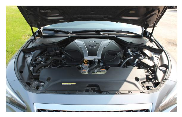
2. The engine cover is held in place with four rubber grommets, one near each corner. Gently pull up as close as possible to each grommet until the cover comes free. Avoid pulling on the very corners of the cover or it could crack.
