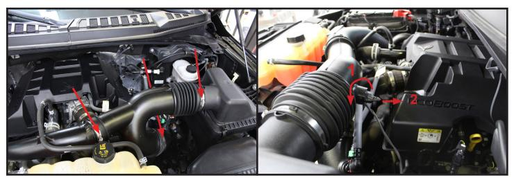
1) Loosen the three hose clamps securing the airbox y-pipe to the OEM turbo inlet tubes and remove the sensor in the y-pipe by rotating counterclockwise about 1/4 turn then pulling out
