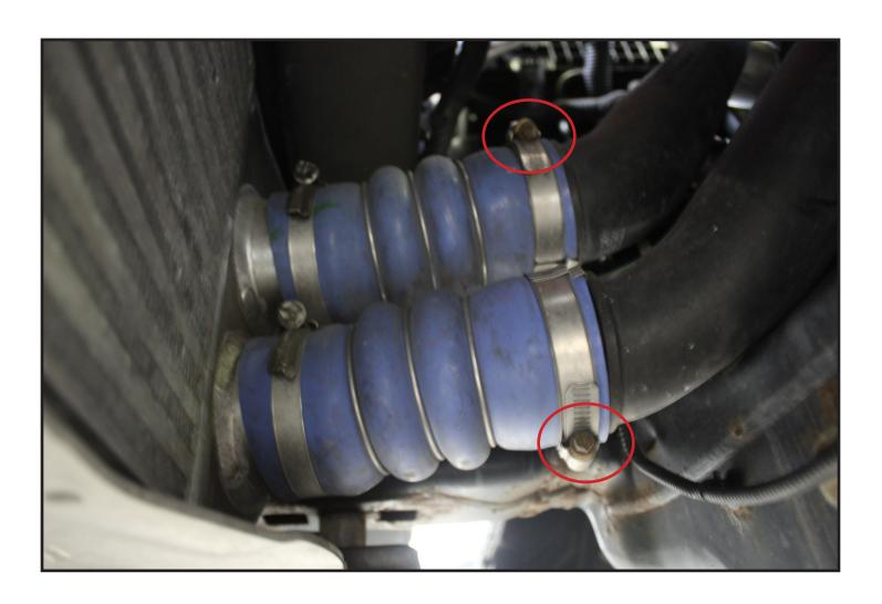
8) Loosen the other end of both charge pipes which are underneath the right side of the front bumper
