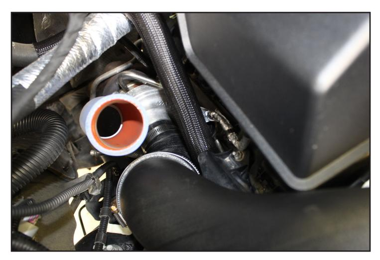
15) Place the right AMS Turbo Inlet Tube into position and orient as shown. Align the right AMS Turbo Inlet Tube silicone and seat the silicone onto the turbo inlet. Use a twisting motion while applying force towards the turbo to seat the silicone to the turbo inlet.
