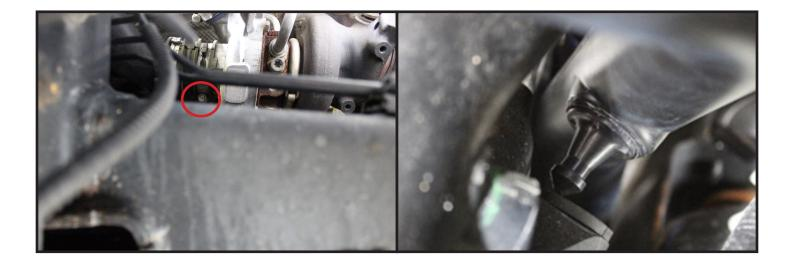
5) From the left front wheel well, use a long screwdriver or 7mm socket with extensions to loosen the hose clamp on the left tube. Next, pull the tube towards the airbox to release the mounting stanchion from the grommet.
