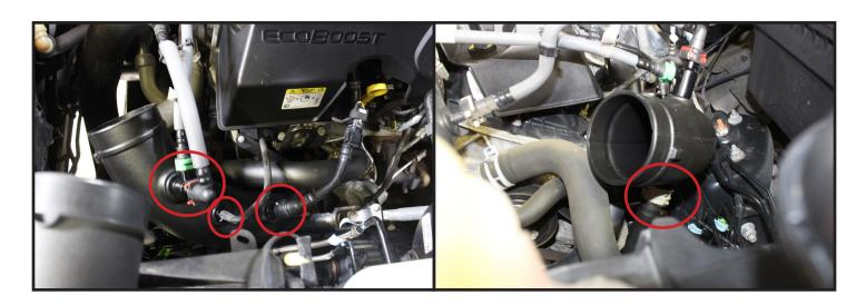
18) Reattach all hoses and fittings (1x green clip, 1x red clip, PCV hose, vacuum hose, and bypass valve return hose)
