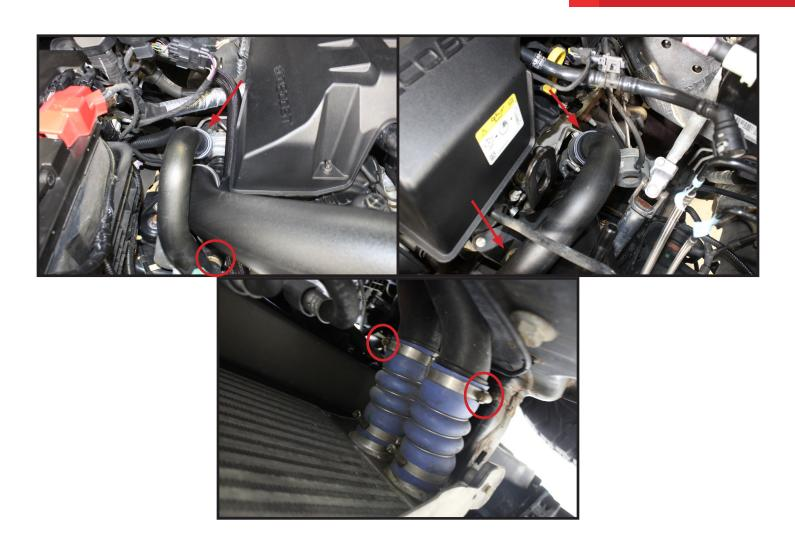
17) Reinstall left and right charge pipes. Make sure to tighten the hose clamps to the same specifications as listed for the other hose clamps. Additionally, ensure that the charge pipe stanchions are properly seated in the grommets.
