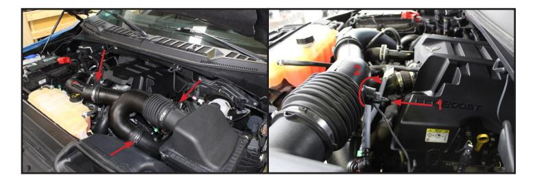
19) Reinstall the OEM y-pipe and reconnect the sensor. Before tightening the hose clamps on the y-pipe, check for proper alignment of the tubes. If necessary, the hose clamps on the AMS silicone couplers can be loosened to adjust the positioning of the tubes then re-tightened once the desired alignment is achieved. Once you are satisfied with the alignment, tighten the y-pipe hose clamps to the same specifications as the other hose clamps.
