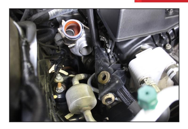
12) Once released, pull the tube from the turbo and remove from the engine bay
