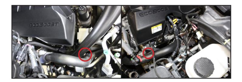
9) Remove both charge pipes. Like the intake tubes, these are mounted with stanchions. Be careful to pull the stanchions out of the grommets when removing the OEM charge pipes.
