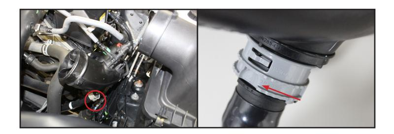
4) Remove all fittings and disconnect the bypass valve return hose. To disconnect the bypass valve return hose, release the quick disconnect by rotating the grey connector in the direction of the arrow shown while pulling away from tube.
