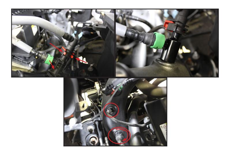
3) Disconnect the fittings shown from left (Driver's side) OEM turbo inlet tube. The green quick disconnects can be released with a flathead screwdriver. The red quick disconnect is released by pinching the lower legs together. Use pliers to remove the spring clamp on the vacuum line (middle). To remove the PCV fitting, pull the silver tab clockwise then pull the connector off vertically at the same time.
