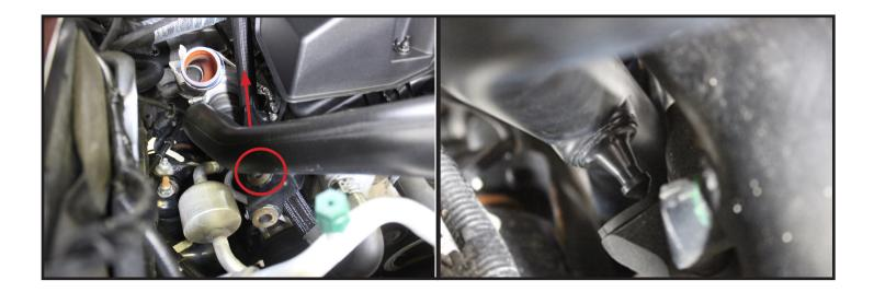
11) Use moderate force to pry the right turbo inlet tube in the direction of the arrow to release the tube mounting grommet. Mount location is underneath circled area.
