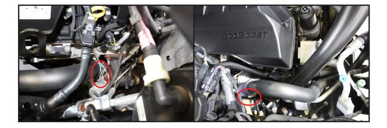
7) Loosen the hose clamps on the turbo ends of both the left and right charge pipes.
