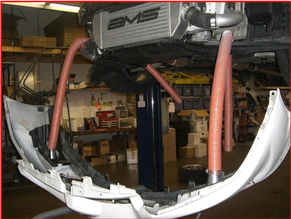
9. With the scoops in place, now you can run the hose through the engine bay and reinstall the bumper cover. To run the hose through the passenger side, most installs will require trimming the plastic oil cooler shroud. The factory undertray will also need to be trimmed to allow the hoses to reach the calipers. Make sure to zip tie the hoses effectively to keep them from touching any moving components (A/C compressor pulley, axles, control arms, etc) and away from very high sources of heat.
