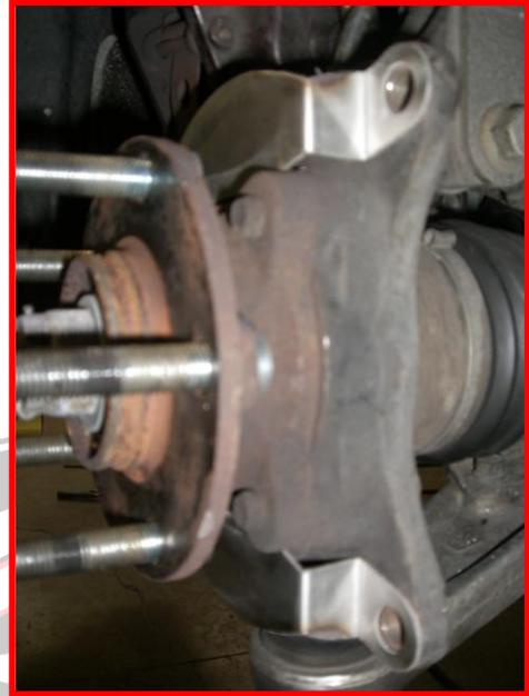
3. Reinstall the rotor. Install the included caliper duct adaptor while bolting the caliper back into place using the factory hardware. Using the supplied coated stainless steel reusable ties, secure the ABS sensor wire to the hub as shown to keep it from rubbing the rotor or touching the caliper (we ended up trimming about 1" from the length of the tie so it wouldn't rub the axle or CV boot).
