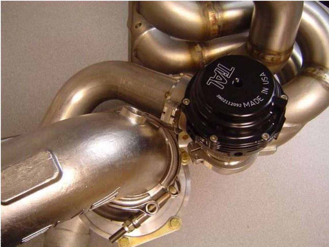
2. Temporarily install the turbo kit. This is done to clock the compressor cover and check clearance around the turbo kit. The best way to do this is with one nut on the top of the header flange and one on the bottom. Then down below bolt the support bracket to the block, on some cars the hole that is used with the support bracket may need to be cleaned out, if that's the case use a M10x1.25 tap to clean up the threads and blow out with compressed air.
