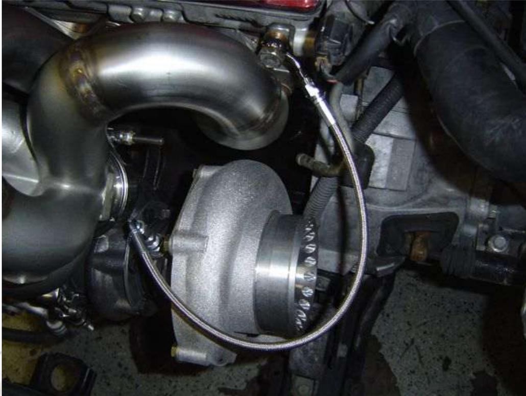
7. Loop the coolant lines using the supplied silicone hose.
