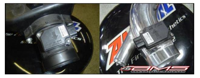
8. Install the air filter onto the AMS intake pipe and install the intake pipe running the MAF sensor wire underneath the intake and connecting it. (If you bought the cold air intake kit you will not be installing the air filter at this time.)
