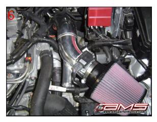
9. Flip the line going from the valve cover to the intake and connect it to the intake pipe. Also at this time connect the line going to the boost control solenoid. The connections are circled in green below. (If you bought an intake without bungs this step does not apply to you, instead you will run the valve cover line to a catch can and install your boost controller at this time.)
