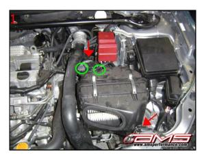
3. Remove the blow off valve, blow off valve tube and the blow off valve vacuum line.
