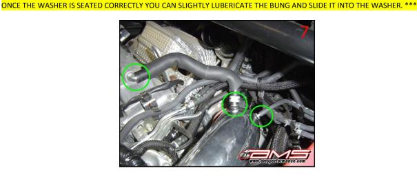
10. Install the blow off valve using the supplied silicone couplers and connect the supplied extended vacuum line.
