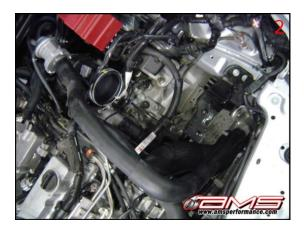
4. Disconnect the line that runs to the valve cover and the line that runs to the boost control solenoid from the intake tube. Loosen the clamp that holds the intake tube to the turbo and remove the intake tube.
