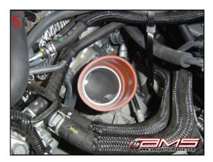
7. Remove the MAF sensor from the OEM intake and install it onto the AMS intake using the supplied screw. Be sure to note the direction of airflow when installing the sensor. The factory screws for the sensor are T25 Torx.
