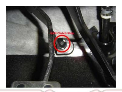
2. Install the adjustable clutch stop and adjust as instructed in the clutch install instructions. Once it is adjusted it can be removed and the additional length of the threaded section can be cut off for a cleaner look.
