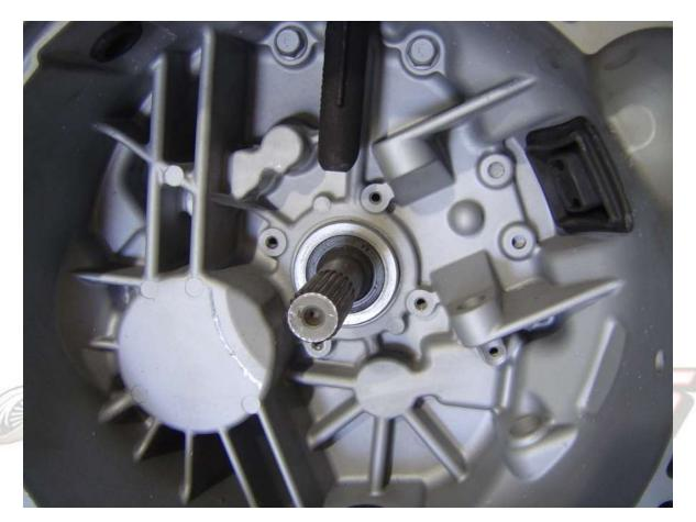
3. Clean off area around the TOB sleeve. Bolt AMS adapter with **both included shims underneath it** to bell housing using supplied hardware and loctite. Make sure to pay attention to the direction of the plate. (The open window of the adapter should face towards where the clutch fork was as shown below)
