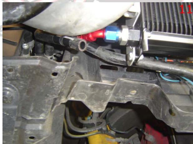
10. Now remove the cooler from the car and push the fittings onto the hose and clamp tightly <sup>12</sup>. The fittings fit very tightly into the hose, heating the hose up helps it to expand and fit over the fittings, a little transmission fluid on the barbs will also help the fittings slide in easier. The 120 degree fitting goes on the longer/top hose, the 45 degree fitting goes on the shorter/lower hose.
