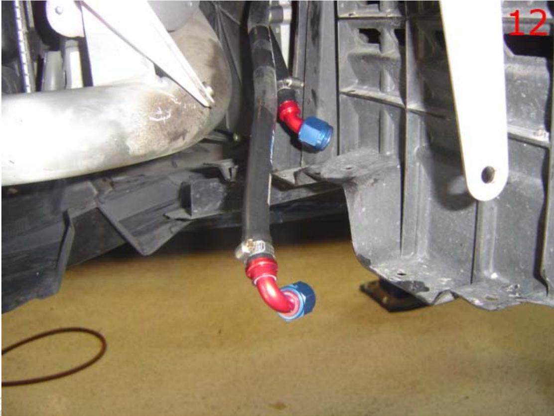
11. Now install the oil cooler <sup>13</sup>. Connect and tighten the lines.
