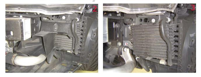
5. Place a clean container under the transmission cooler <sup>4</sup>, disconnect lines and let them drain into the pan. You MUST catch all fluid and put it back into the transmission when done, there is no way to measure the fluid level in the transmission. You can now also remove the transmission cooler and drain all of the fluid from it into the pan also, make sure not to get any dirt or debris
