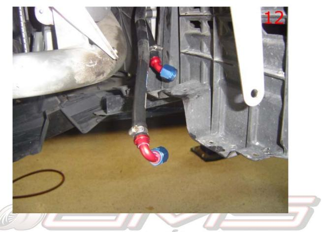
11. Now install the oil cooler <sup>13</sup>. Connect and tighten the lines.
