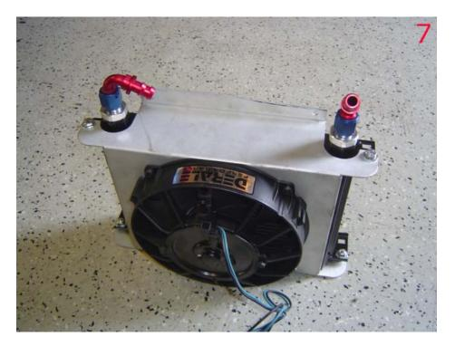
8. Now loosely install the cooler and cut the hoses so they can be pushed onto the fittings while still allowing enough movement to not put tension on the hose. The long hose goes to the top fitting. In most cases the longer hose will be cut about 2.5" closer to the transmission from the heat shield on it <sup>8,9</sup>. On the short hose cut right after the slight bend in the hose <sup>10,11</sup>. Variances are always possibly, double check before cutting.
