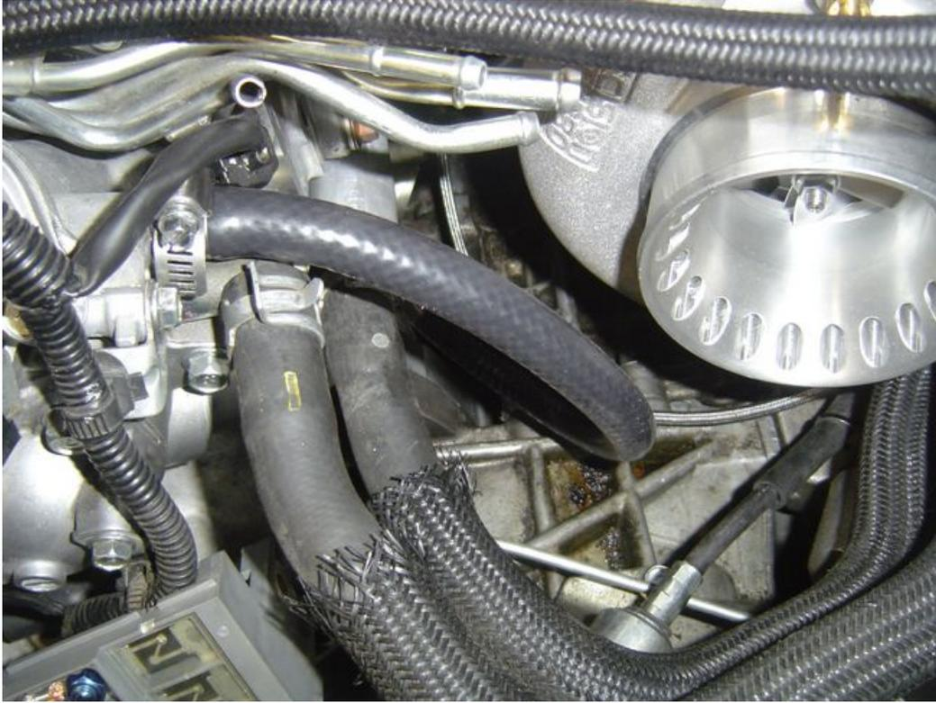
21. Install supplied heater hose on AC line that is on the firewall.
