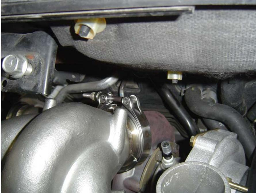
16. Install downpipe and once all connections are lined up tighten the downpipe to the exhaust connection, the downpipe to turbine housing connection, the turbine housing to the exhaust manifold connection and finally the support bracket mount.
