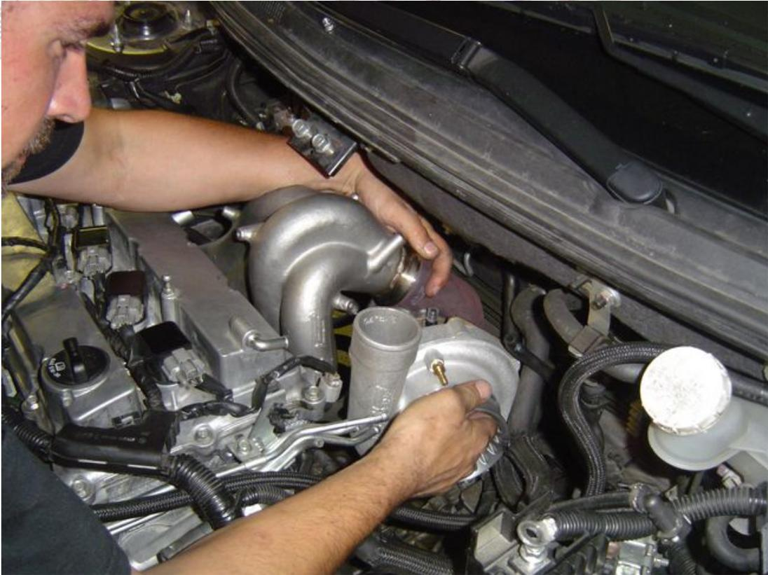
14. Take a look at the support bracket where it bolts to the factory bracket. IF there is a space in between the two this space must be filled with the supplied thick M12 washer, this must be done to ensure the support bracket will not be getting pulled down. Install the nylock nut and bolt at bottom of support bracket to hold the assembly in place. Leave loose for now to allow movement of the turbo.
