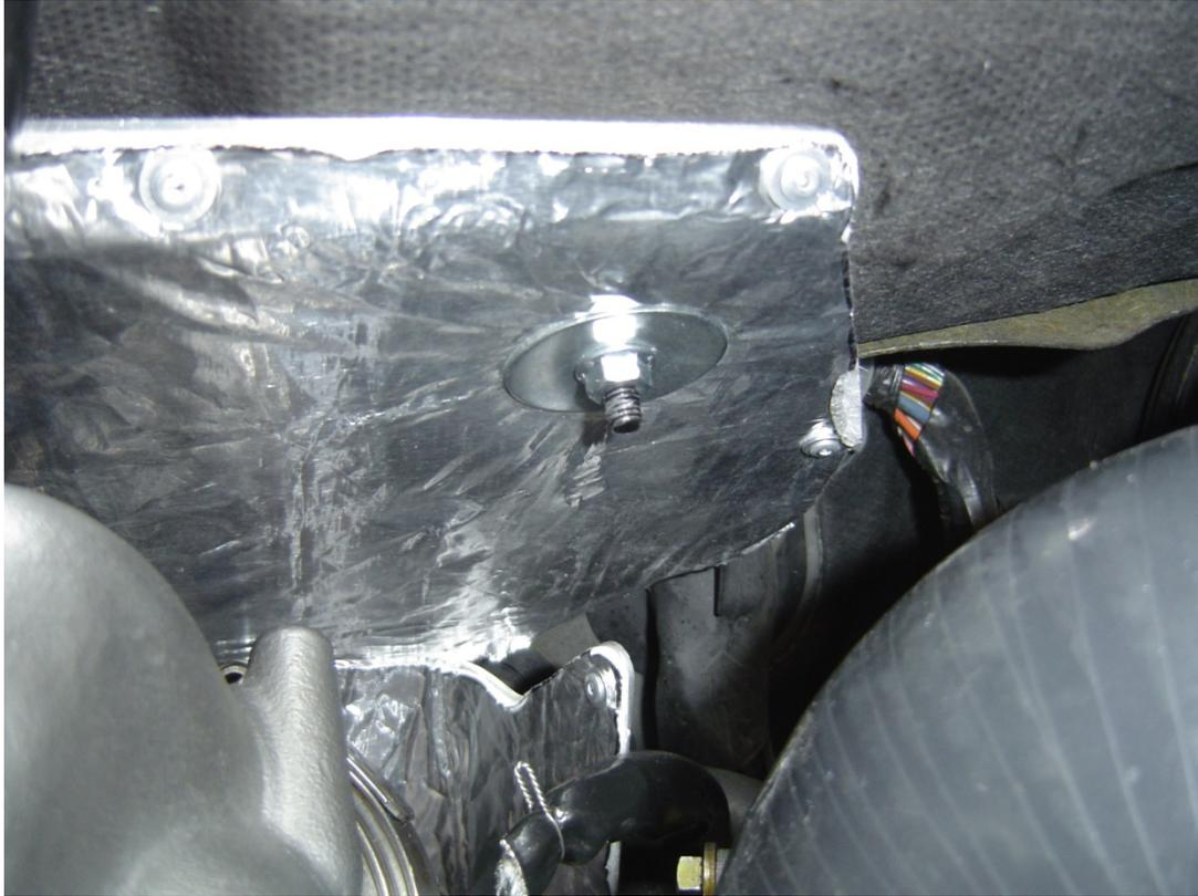
23. Install manifold shield.
