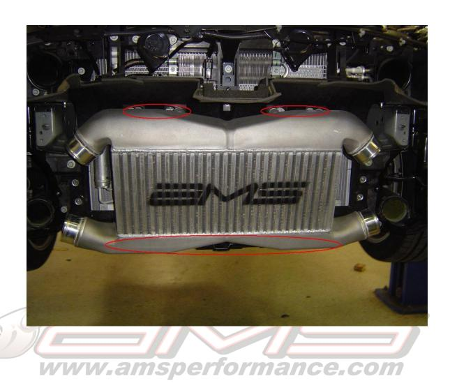
14) Re-install intercooler shroud using 4 supplied 6x12mm bolts and nuts where plastic rivets were cut out.
