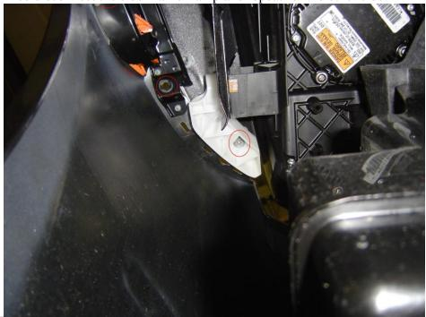
5) Remove 6 clips holding top of bumper to radiator support and carefully remove bumper. Disconnect fog lights if equipped.
