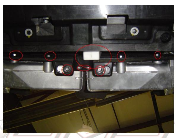
12) Begin removal of factory intercoolers by removing 2 8mm bolts at top of each intercooler. Move to bottom of intercoolers and remove 2 rear facing 8mm bolts in lower intercooler end tanks. Remove 8mm bolt from bottom of intercooler end tank. Repeat these steps for 2<sup>nd</sup> intercooler. At this point the intercoolers should come free of the car.
