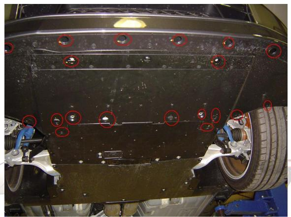
3) Remove front section of inner fender liners. 9 clips and 1 screw per side.
