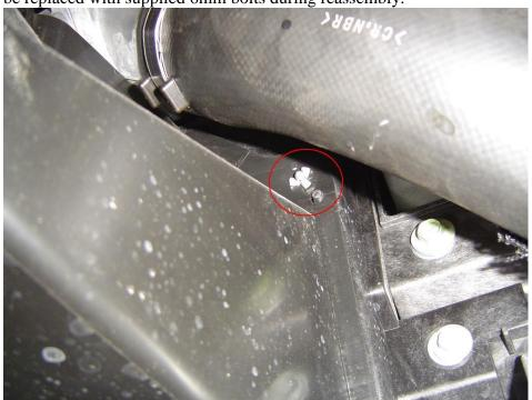
9) Remove oil cooler ducting by removing 4 clips.
