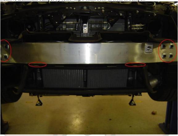
8) Cut 4 plastic rivets off of the intercooler shroud and remove shroud. These will be replaced with supplied 6mm bolts during reassembly.
