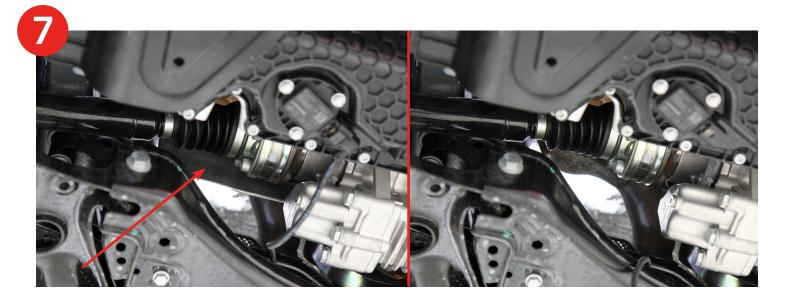
8. Remove the heat shield around the transfer case output shaft. It is held in place by a 10mm triple square shown in the picture and a 16mm stud bolt on the side where the shield in step # 7 was removed.
