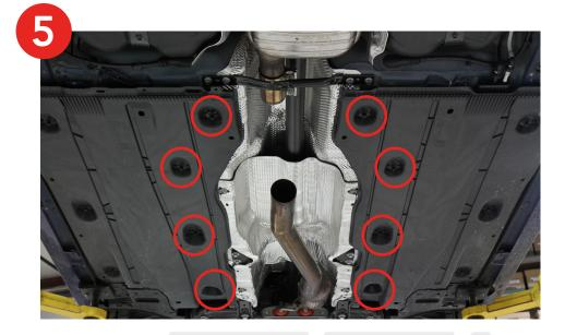
6. Next step will be to remove the center exhaust heat shield to expose the driveshaft. To do this, use needle nose pliers to grab on to the four metal retaining washers and turn counter clockwise while pulling downwards. There will be little triangle cutouts on the washers. The trick is the push in two of them 180 degrees apart with the pliers and grab it from there.
