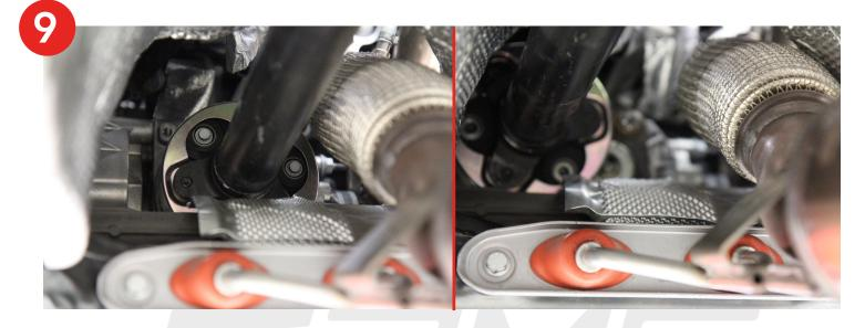
10. Remove the heat shield on the subframe. It is held in place by four T30 Torx bolts. Removing this heat shield will help when removing the factory downpipe and installing the new AMS downpipe without bending the shield.
