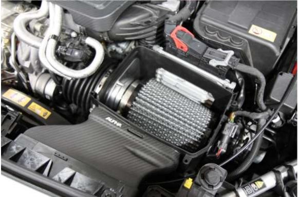
11) Install the Carbon Air box lid using the factory screws that you had set aside earlier.
