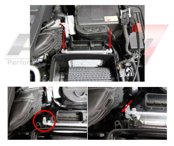
5) Loosen Hose Clamp between air box and turbo inlet hose.
