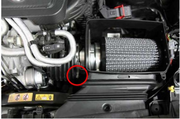
6) Now that the ECU has been removed and the hose clamp loosened, you can now lift up on the air box in order to remove the factory air duct.
