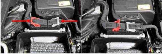
4) Remove the ECU by un-clipping the two spring retainers shown and then pull upwards.
