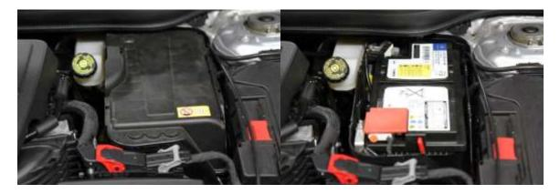
2) Remove the air box lid by loosening the four T25 Torx screws. Remove the screws from the lid and set them to the side to be reused.
