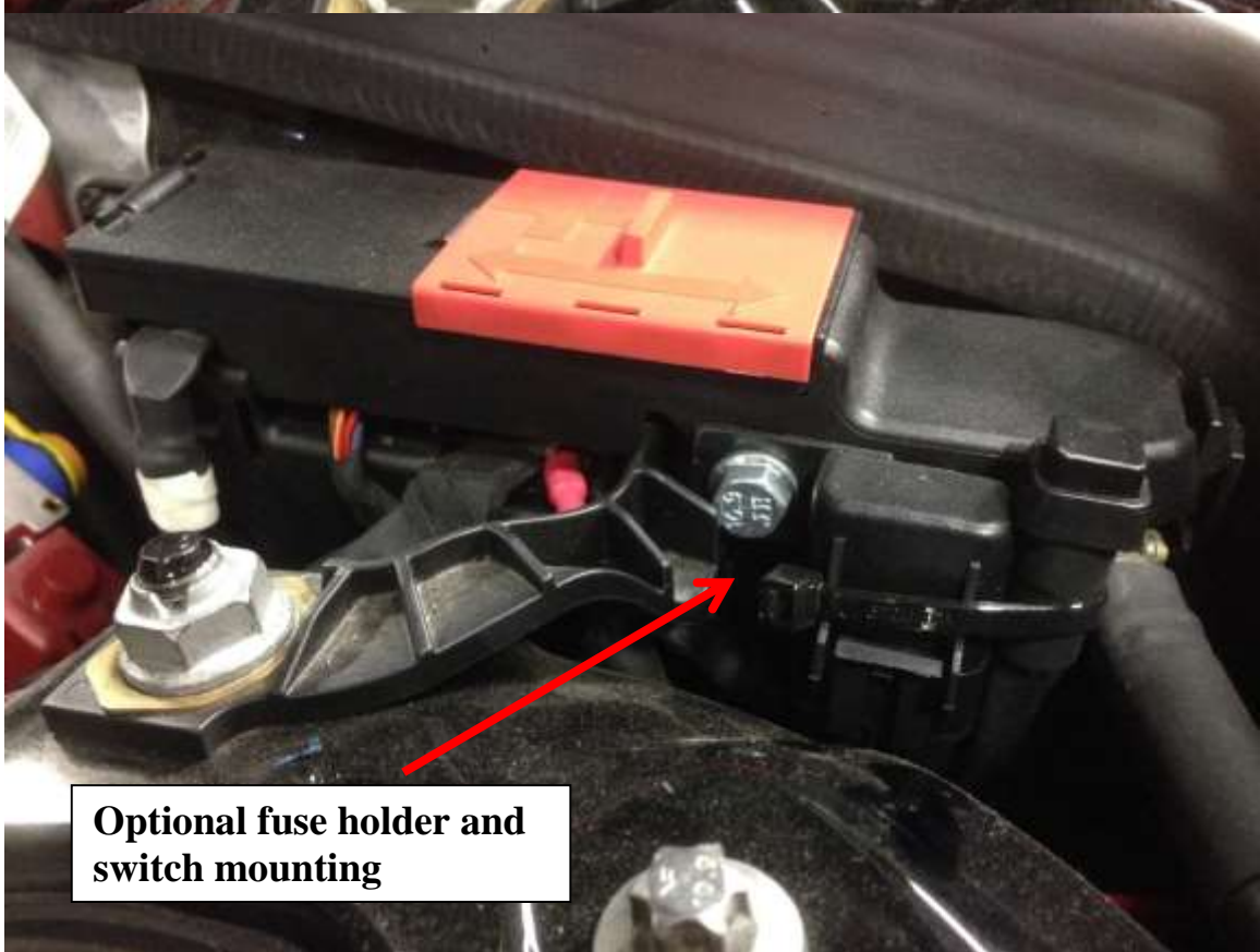
Wire harness power wire connection
