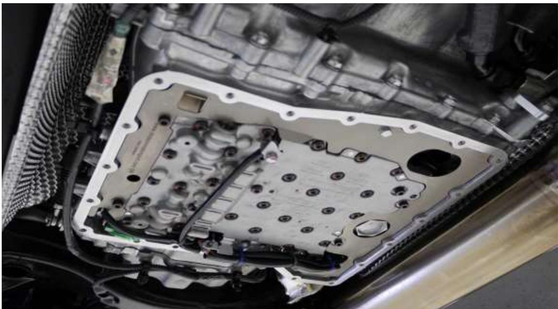
10. Apply sealant (we recommend Three Bond #1217H) to the top sealing surface of the pan spacer included in the Alpha kit. Spread evenly around bolts.
