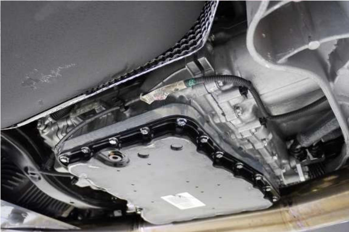
16. Wait at least an hour for the sealant to cure fully before re-filling the transmission. This will improve the sealing qualities of the silicone and reduce the possibility of leaks.
