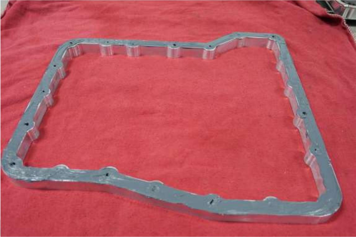
11. Install spacer onto transmission using included M6 bolts. Snug the spacer onto transmission to set sealant. Wait at least a half an hour to let the sealant cure enough to hold the weight of the spacer.
