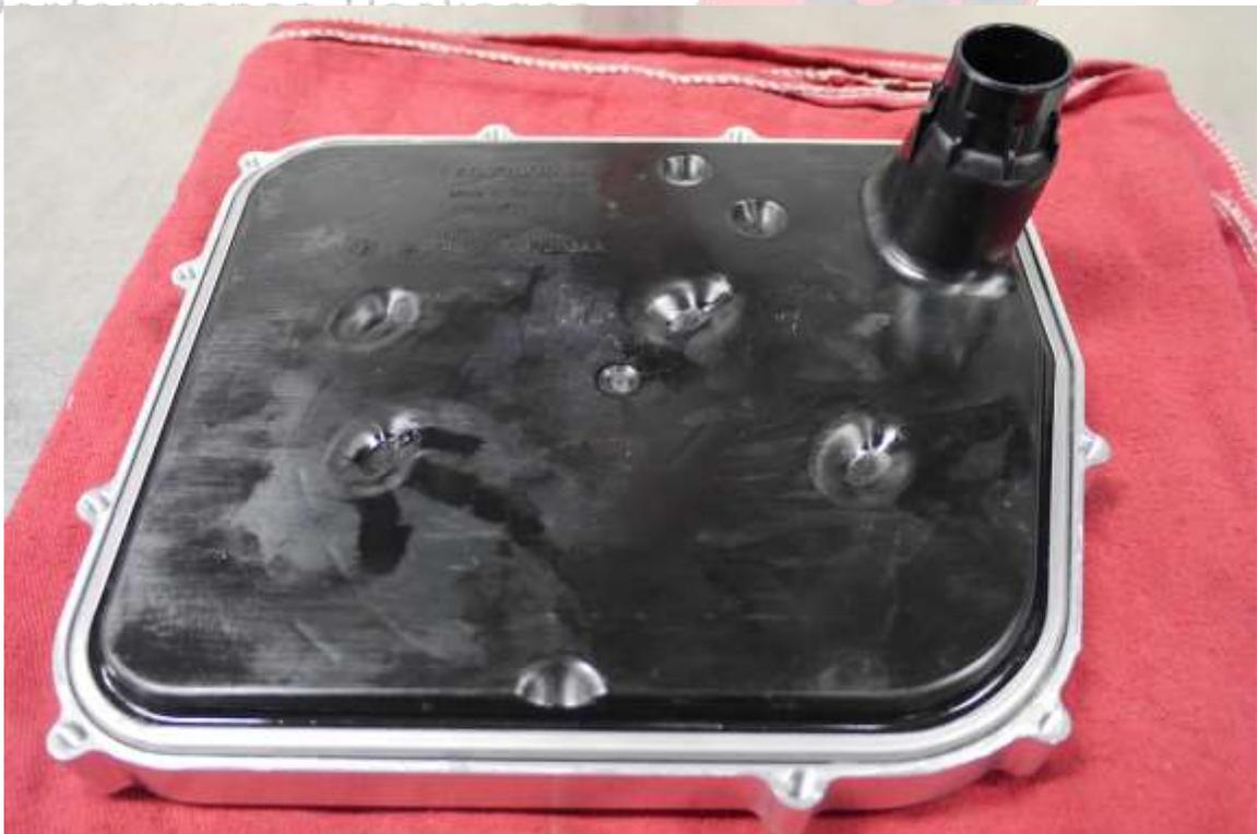
7. Install Alpha retaining ring as shown using the included M6 button head screws. Use high temp/strength thread locker. Torque to 90 in/lb
