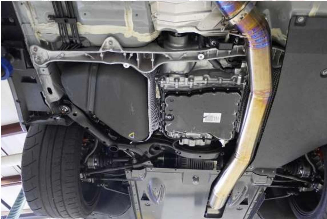
2. Drain transmission by removing factory drain plug and level straw.
