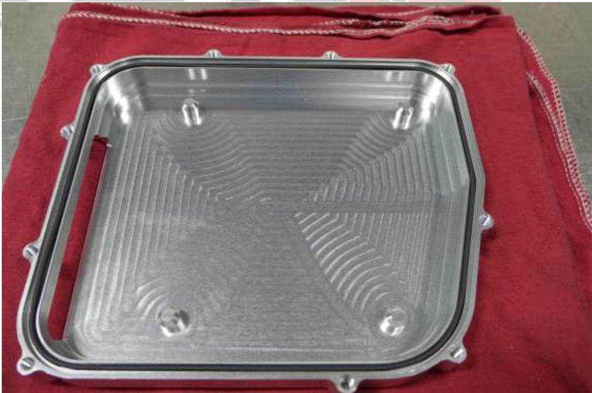
6. Install factory filter/pick-up into the Alpha billet housing as shown. NOTE: The fit is tight and may require some light force to seat it all the way into the pickup. Also, it is important that the o-ring stays in its seat/groove.
