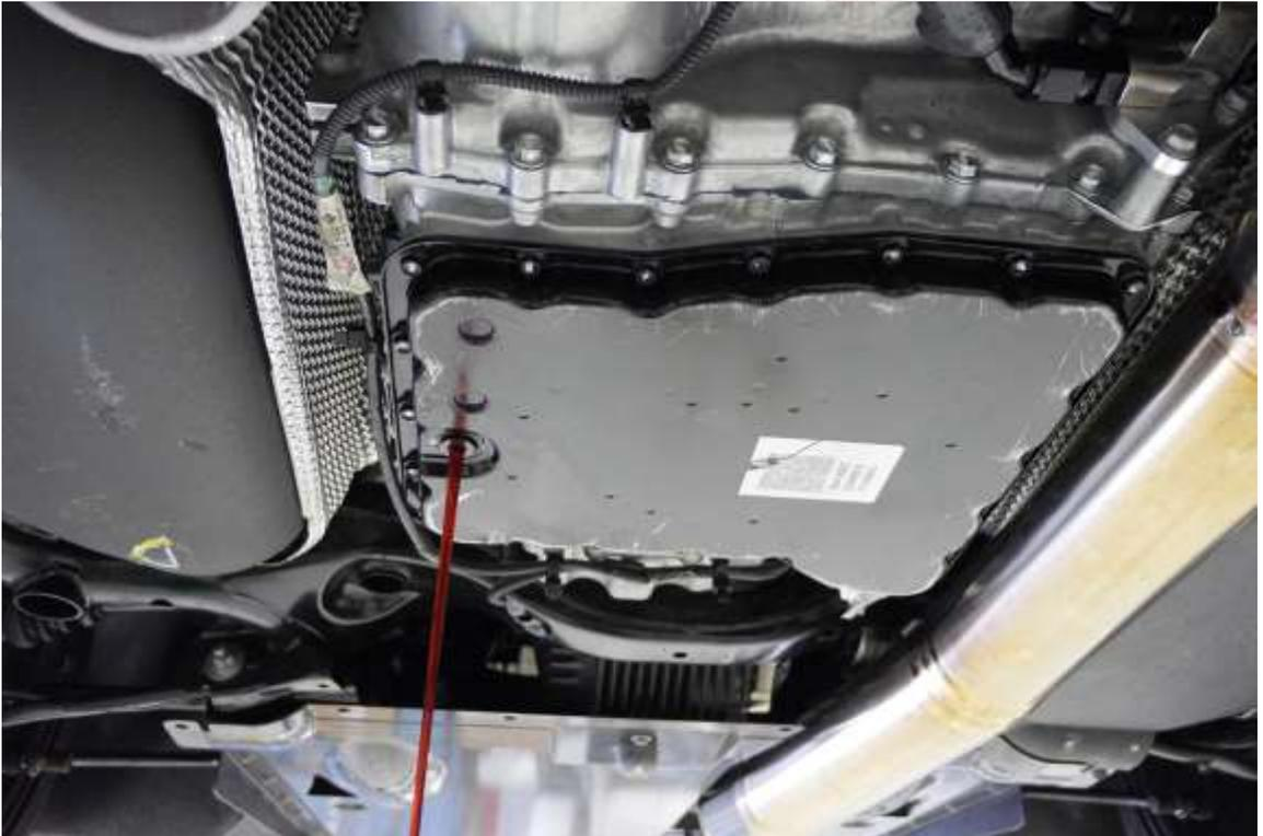
3. Remove transmission oil pan by loosening the M6(10mm head) bolts around the perimeter. Support the pan while removing as it can fall. NOTE: There will be some fluid remaining in the pan even after draining.
