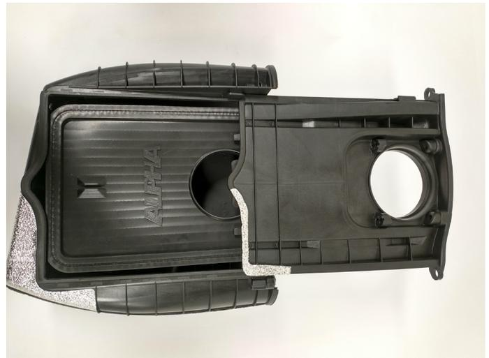
02. Slide filter housing cover onto the filter housing until it is in place. Some downward pressure may need to be applied to the filter so that the features on the filter housing cover clear the edges of the filter.
