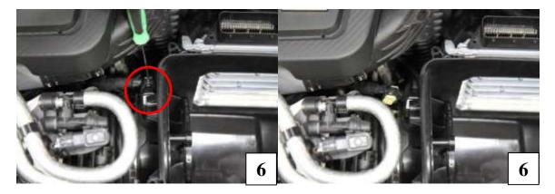
7) Loosen the hose clamp on the coupler to air box connection using a 7mm socket or flat head screw driver. Pull the air box inlet towards the front of the car away from the air box. Pull up on the air box assembly to remove it from the car. It is held in place by three rubber grommets under the air box. The air box inlet will remain in the car.
