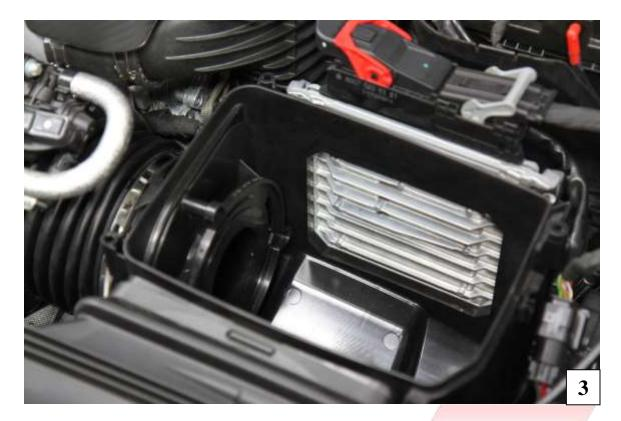
4) Remove the connector and wire harness on the side of the air box. To remove the connector, release the tab on the air box and slide the connector down and out of the way. The wire harness clip will just pry off the air box using a flat head screw driver.
