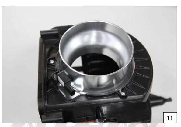
11) Bolt the new Alpha Intake into the factory air box using the three supplied m5 button head bolts.
