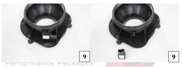
10) Install the MAP sensor into the new Alpha Billet Intake in the reverse order of removal during step 9).
