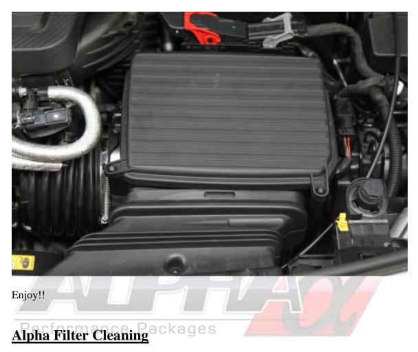
15) Reinstall the air box lid. Reconnect the battery and reinstall the cover. Double check all the connections are complete.
