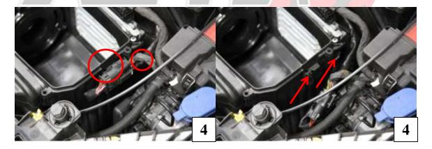
5) Disconnect the ECU by releasing the Red and Grey connector levers. Pull the connectors off to the side.
