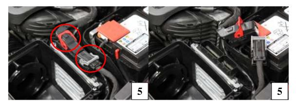
6) Disconnect the MAP sensor on the air box. To do so, use a small screw driver to pull out the grey tab from the connector. Once released, depress the grey tab down to disconnect.
