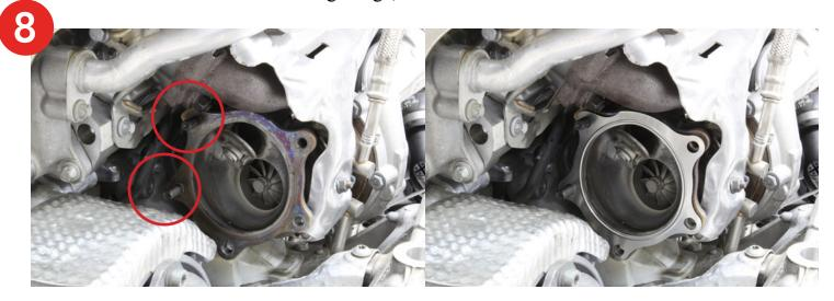
**9.** Install the new Alpha turbine outlet side of the downpipe using the new supplied nuts. Reinstall the mounting bracket bolt.
