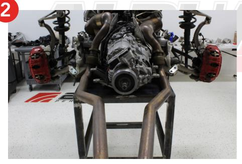
**3.** Remove all four O2 sensor for the factory downpipes
