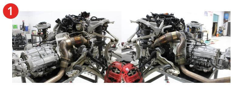
2. Remove the mid pipes sections. The right downpipe connecting studs are facing upwards and are easiest to remove with the engine down.
