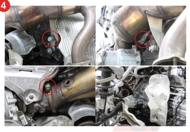
**5.** Install the assembled left side Alpha downpipe in the reverse order of removal. Use the supplied M8 nut for the backside of the spring bolt. Reinstall the O2 sensors.
