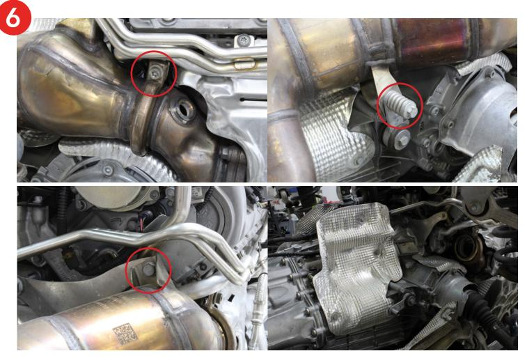
7. Next remove the second part of the downpipe. Unbolt the piece from the turbine outlet flange. If the studs come out with the hardware, this is ok as some studs will need to be removed to install the Alpha downpipe.
