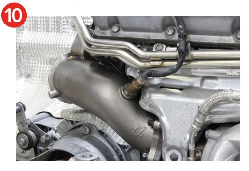
11. Install the second half of the downpipe using the new supplied V-band clamp and reusing the spring bolt. Clock the V-band bolt as shown below. The stud should be facing upwards towards the inside of the engine. Use the supplied M8 nut on the back side of the spring bolt.
