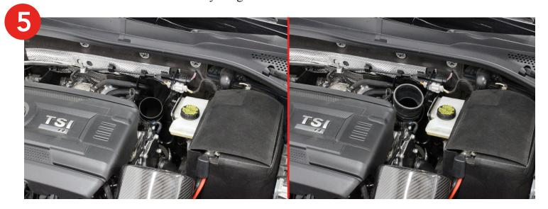
**6.** Slide the intake tube in place. Make sure the isolator grommet is fully inserted into the carbon air box. Failure to make sure the isolator is fully inserted could result in the isolator pulling out of the air box. The intake tube will sit further into the air box to allow the engine to rotate backwards giving the isolator more movement in the outwards direction. Once everything is adjusted properly tighten the hose clamps taking note of the torque spec listed below.
