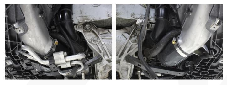
**23.** Locate and install the supplied intercooler outlet silicone coupler. They are labeled left and right. Use the #36 and #44 hose clamps provided. Adjust as necessary. Reinstall the factory plastic charge air y-pipe mounting bolts.
