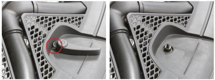
**03.** Remove the four retaining clips from the core support cover. Lift upwards at the front and remove the cover panel front the vehicle.
