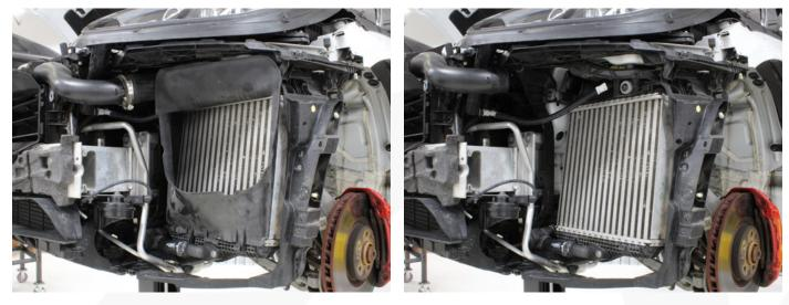
14. Disconnect the bypass value at the hose connected to the intercooler. Release the quick connect fitting on the factory inlet coupler at the bottom of the intercooler. Remove the three bolts holding the intercooler to the frame and remove the intercooler assembly. Repeat the process for the other side.
