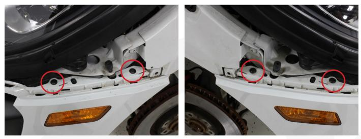
11. Remove the four Torx screws from the top of the bumper. Carefully remove the front bumper.
