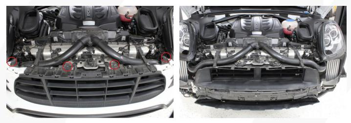
**12.** On the front louvered air duct, the side are on hinges. Release the tabs and rotate the sides towards the front. Remove the five bolts holding the plastic charge air y-pipe in place. The y-pipe will not be removed but will need to be moved around to remove and install the silicone couplers.
