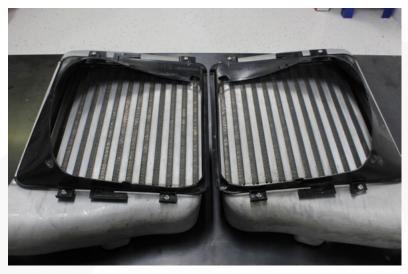
**19.** Remove the bypass fittings from the front of the factory intercoolers. Use the supplied M6x12 bolts and install the fittings on to the Alpha intercoolers. Do not reuse the factory screw in the Alpha intercoolers.
