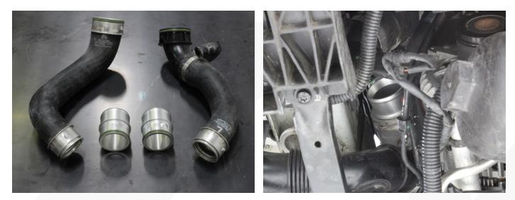
17. Locate and install the supplied compressor outlet / intercooler inlet silicone couplers. Use the supplied #32 hose clamps on the compressor outlet adapters and the #48 hose clamps on the intercooler inlet side. A #8 hose clamp was supplied for the PCV hose connection on the left side. There is very little room on the left side so adjustments will need to be made when connecting the intercooler when installed.
