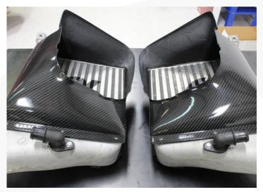
**21.** Install the intercoolers using the supplied M6 x 35mm bolts to mount the intercoolers. Do not reuse the factory bolts as they are too short. Connect the bypass valve hose when installing.
