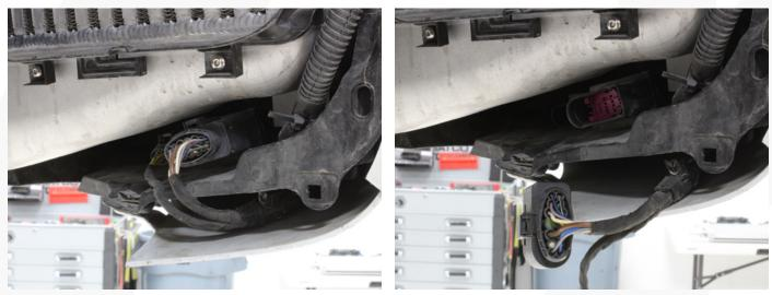
**09.** Remove the two Torx screws just inside the wheel well area securing the bumper to the frame on each side.
