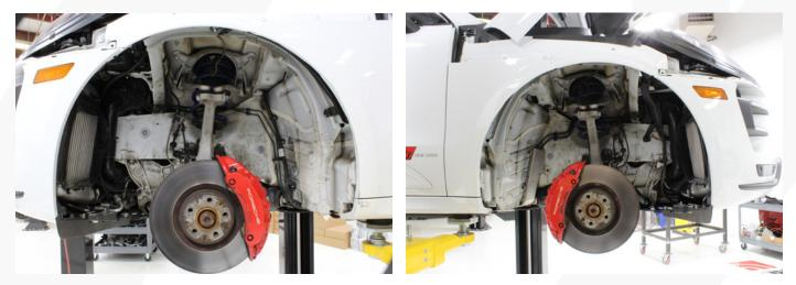
**06.** Raise the vehicle and remove the center under tray. Remove the corner panels as well. There is a water drain hose connected to the top of the panels that needs to be disconnected.
