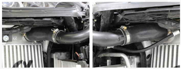
24. Last, install the carbon ducts. Use the provided M5 hardware.
