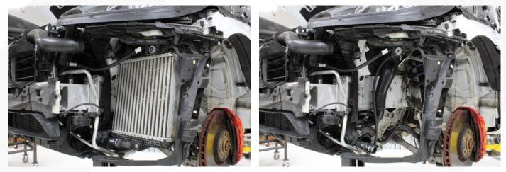
15. Remove the factory turbo outlet / intercooler inlet couplers. Releasing the quick connect clip on the turbo compressor outlet and leave the clip in place. On the left side, disconnect the small hose connected to the intake tube. This is part of the PCV system.
