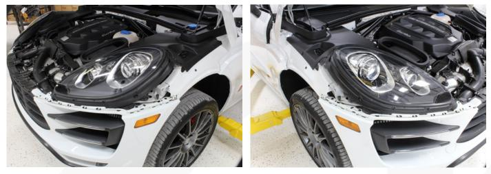
**05.** Remove both wheel well liners. There is also one screw per side that is on the outside of the body that also needs to be removed.
